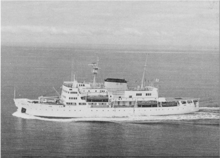
The CSS Baffin is a diesel-driven ship designed primarily for hydrographic survey work in arctic waters. (BIO 2874-29)
