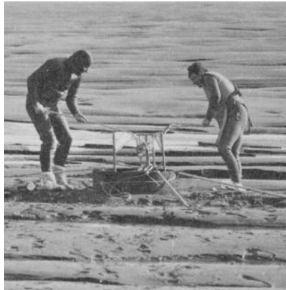
Top: A sand bar in the Minas Basin, NS, photographed by an unmanned balloon-supported camera and depicting the survey pattern used for radioactive tracer studies. Bottom left: a survey vehicle and marker on the bar. Bottom right: radioactive tracer is released on the sand bar.
