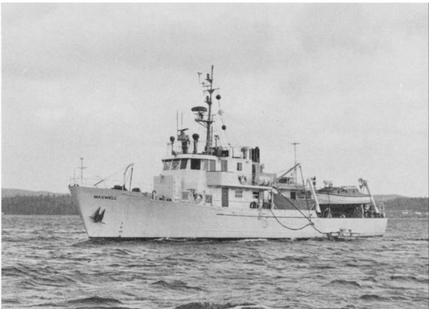
The CSS Maxwell is a diesel-driven ship designed for hydrographic work in nearshore and coastal waters. (BIO 2637-2)
