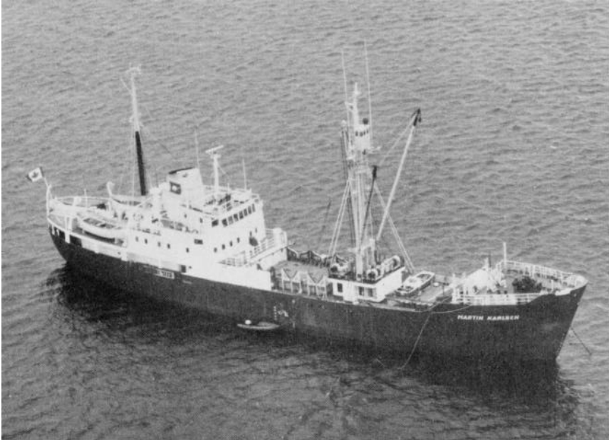
The MV Martin Karlsen is a charter vessel used mainly for hydrographic-geophysical surveys. (BIO 4994-4)
