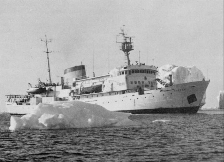
The CSS Hudson is a diesel-electric driven ship designed as a combined oceanographic research and hydrographic survey vessel. (BIO 4926-C-7)
