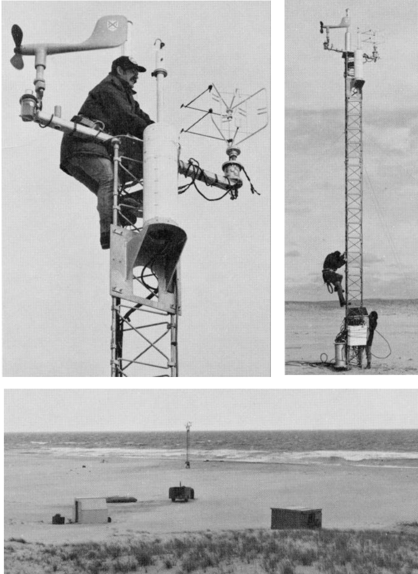
Measurements of air-sea exchange of CO 2 in the waters off Sable Island, NS, October, 1978. Top left (left to right): an aerovane anemometer, a CO 2 sensor, and a sonic anemometer. Top right: the ten-metre tower on the beach. Bottom: tower, generator hut, and data recording shelter. (BIO 5050-52-53, 58)
