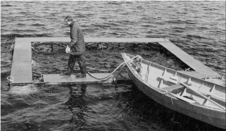
The submersible raft used for shellfish production experiments. (BIO 4740-24)
