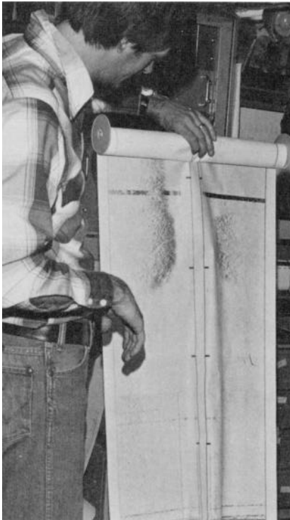
Left: a side-scan sonar survey record, which depicts changes in the sea floor charted over a 1500-metre wide track. Right: the side-scan sonar system is retrieved. (BIO 4978-10-8 and 5007-7-3)
