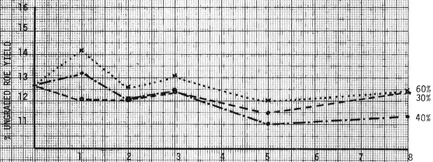
FIGURE 8. EFFECT OF BRINING TIME AND BRINE CONCENTRATION WITH ADDED SORBATE ON ROE YIELD
