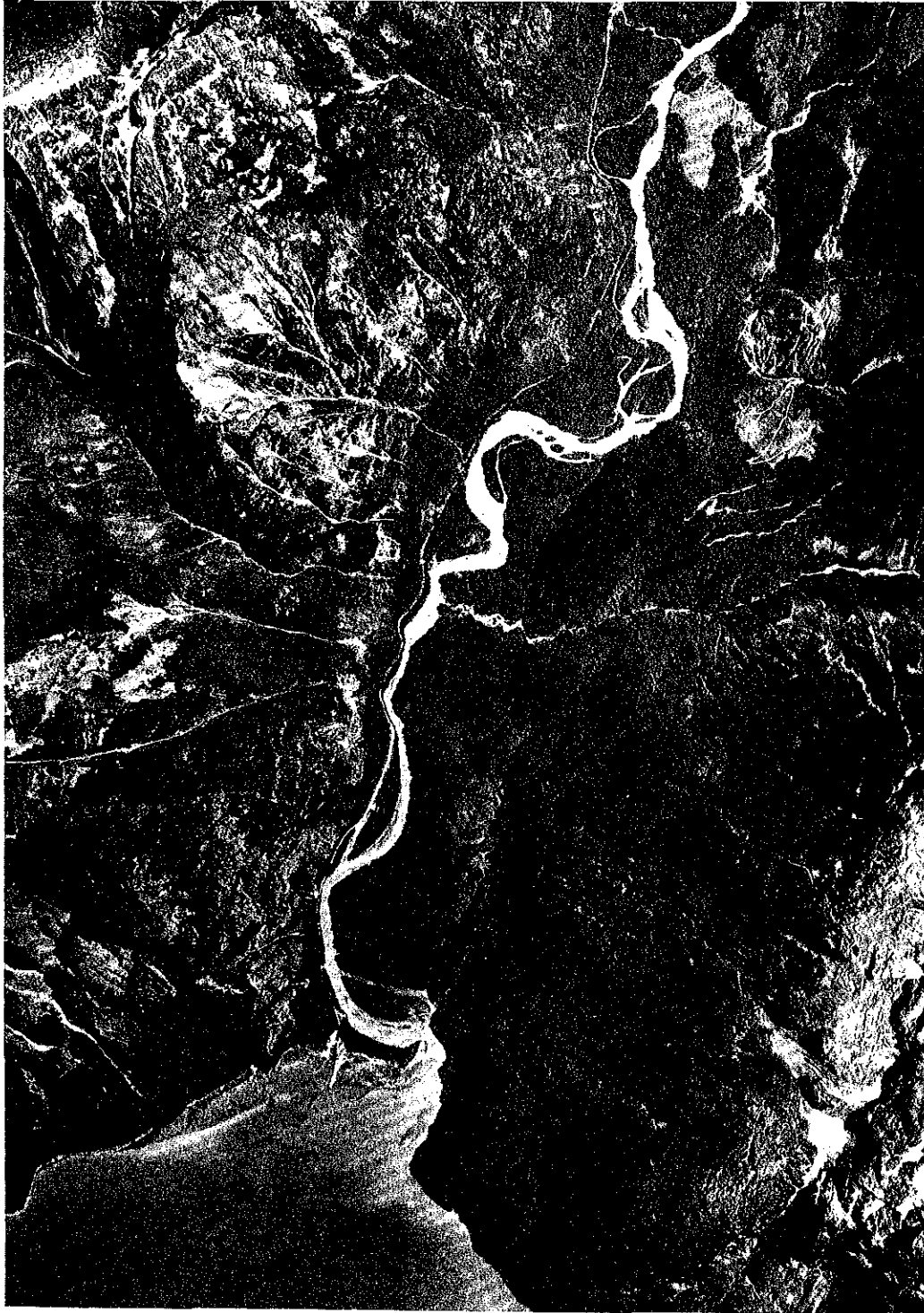
FIGURE 3.1 Lower Southgate River (BC77116: 150). Aerial photograph showing gravel accumulation zone and abrupt transition to a sand bed channel.
