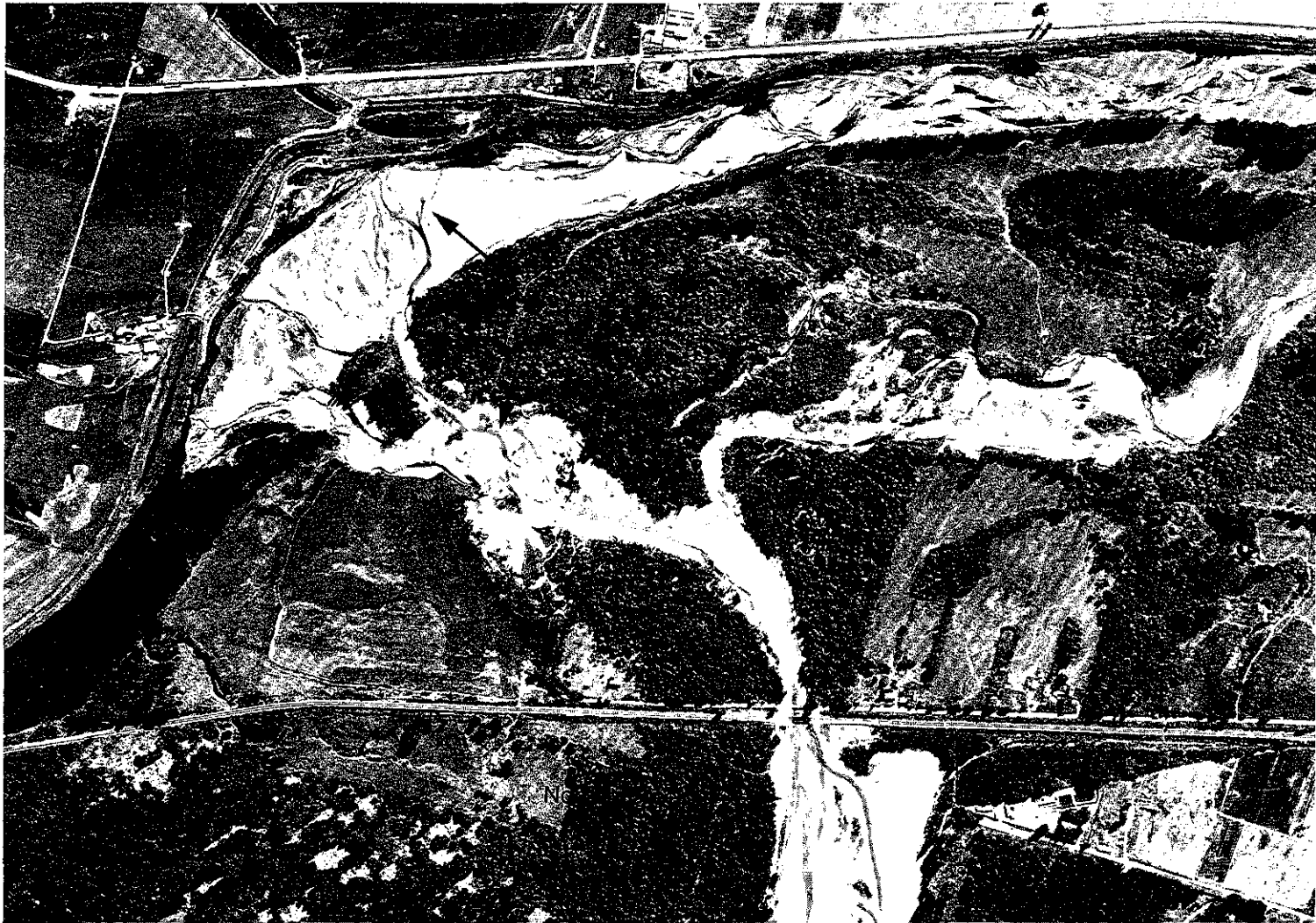
FIGURE 2.2 Norrish Creek (BCC 536:061). Landsliding and accelerated gravel supply and transport in a small basin.
