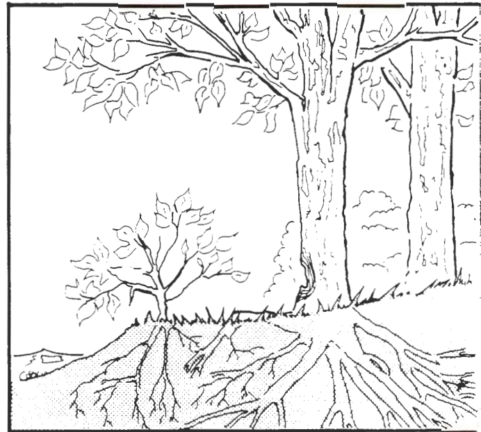
FIGURE B-2: ACTION OF ICE ON BANK VEGETATION IN THE SPRING SHOWING REJUVENATION OF A DAMAGED SHRUB. EVEN WHILE DAMAGED, THE ROOTS OF THE SHRUB STILL RETAIN SOIL, PREVENTING BANK EROSION.
