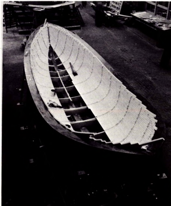
Figure 2. Core-mould system – 26-foot motor surf boat, female forms.
