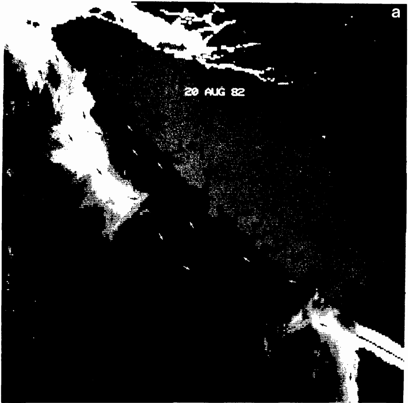
FIG. 13. NOAA satellite thermal images for the west coast of Vancouver Island. (a) 20 August, 1982. Lightest oceanic areas are about 11°C and darkest areas about 15°C; (b) 26 August, 1986. Light = 8°C and dark = 12°C; (c) 12 October, 1986. Light = 7°C and dark = 14°C. Arrows denote direction of flow. The Coastal Current, Juan de Fuca Eddy and wave-like flow perturbations are visible in all images. Relatively cold filaments penetrate southeastward past Brooks Peninsula in summer.
