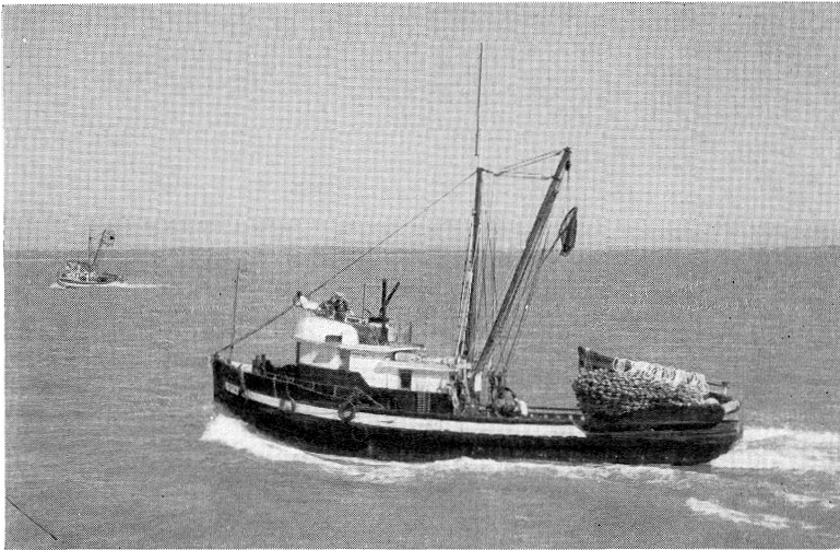
FIG. 17. A Pacific Coast purse seiner. Introduced to the Newfoundland area in 1939. (Photograph by National Film Board of Canada.)
