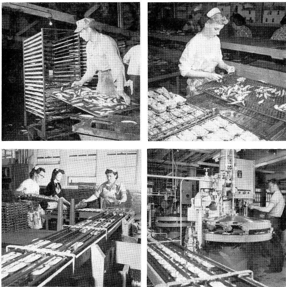
FIG. 4. The interior of a Maine sardine cannery. Top left: Removing sardines from the cookers. Top right: Cutting and packing the fish. Bottom left: A conveyor belt from the packers to sealing machine. Bottom right: A sealing machine.
