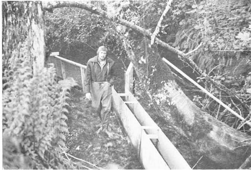
Note that the sluice trough originates at the upstream end of a riffle.
