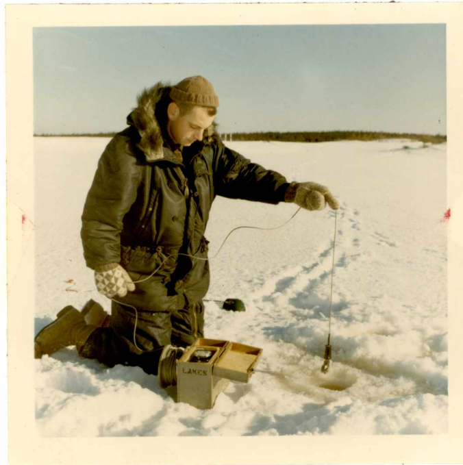
Fig. 11. A simple electric thermistor used to obtain a vertical series of water temperatures beneath the ice at Thomas Pond.
