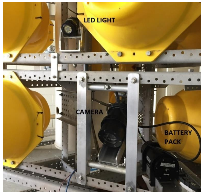
Figure 1. Time Lapse camera system mounted to lander for test deployment.
