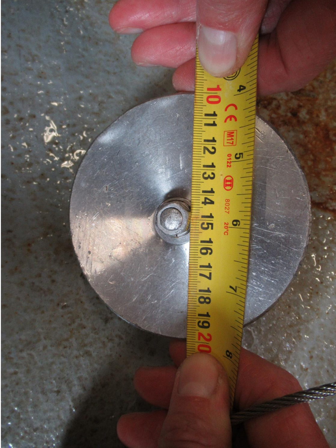
Image of the drop weight used to trigger a photo with the 4K Camera. The weight is 10 cm in diameter and can be used as back-up scale if the lasers are not visible.
