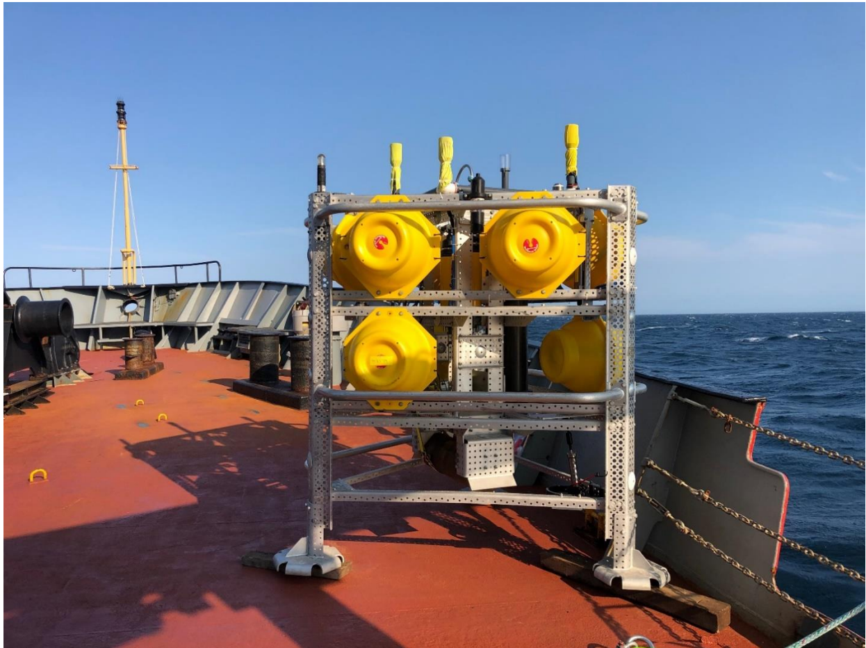
Figure 16. Photo of Lander 3 prior to deployment. The AMAR can be seen (black cylinder) with three hydrophones covered by yellow clothes on the top.
