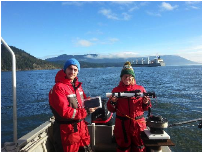
Figure 3: A typical patrol, with team members on the rear deck of their vessel displaying the equipment used. Note the downrigger at right, the CTD profiler being shown by the patrol member at center, and the tablet held by the patrol member on the left.
