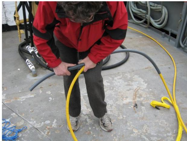
As can be seen in the photo, the woven strain relief is in place and will cover a portion of the hose/umbilical.
