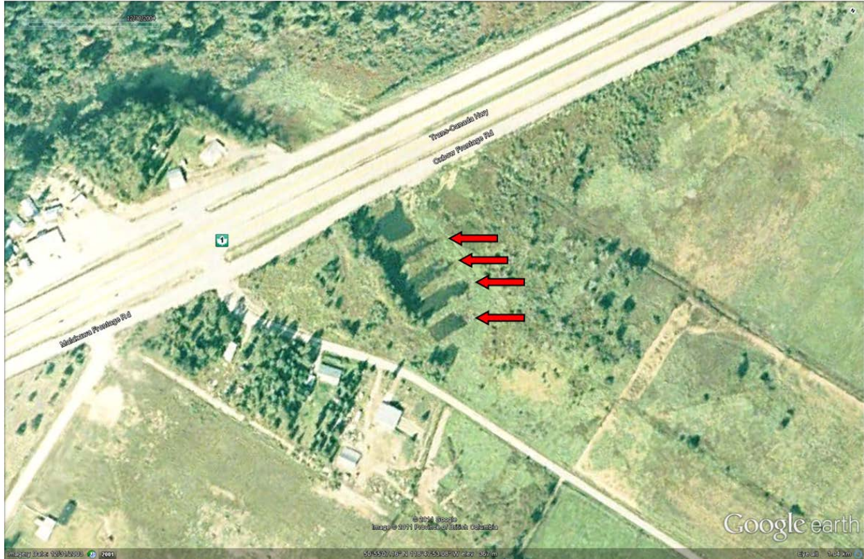
Figure 3. Aerial photograph taken in 2004 of 6 ponds constructed in 1987 as compensation for highway widening near Malakwa BC. Infilling by vegetation and sediment noted by Lister and Bengeyfield (1998) is evident in the 2nd to 5th ponds (arrows).
