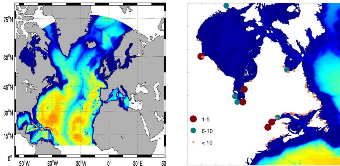
Figure 33. The North Atlantic Ocean model (NAO) domain (left panel). Bathymetry coloured from red (deep) to blue (shallow). The locations of the 45 rivers, colour-coded based on ranked discharge (right panel). The top four rivers are the St. Lawrence, Nelson, Saguenay and La Grande.
