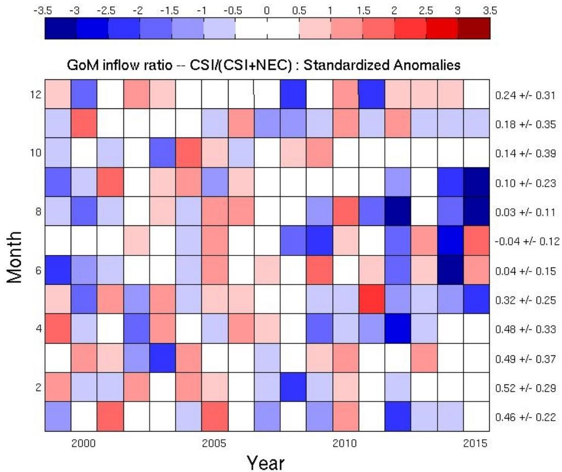
Figure 38. Standardized anomalies of the Gulf of Maine (GoM) inflow ratio for years 1999-2015. Numbers to the right are monthly means and standard deviations. CSI = Cape Sable Island; NEC = Northeast Channel.
