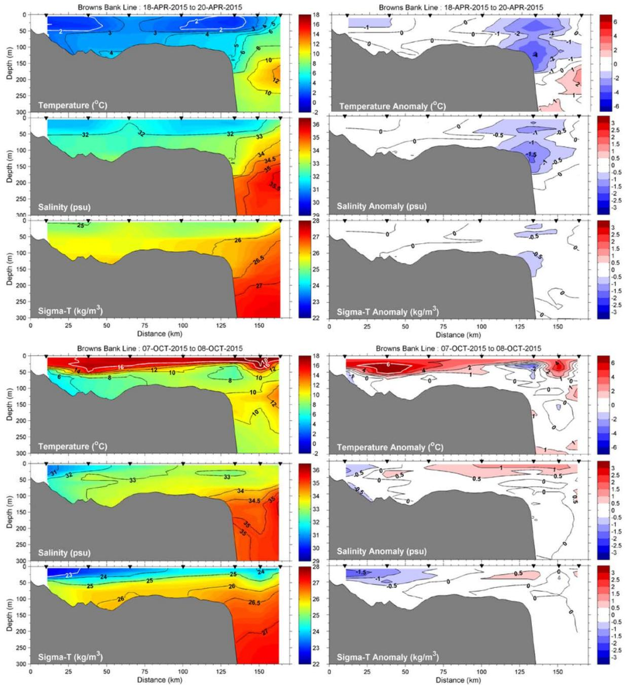
Figure 24. The 2015 sampling of the Browns Bank Line for Spring (top three panels) and Fall (bottom three panels). Temperature (top panel in each group), salinity (middle panel in each group) and density (lower panel in each group) and their anomalies with respect to 1981-2010 monthly means (right panels). Bullets indicate periods of sampling.
