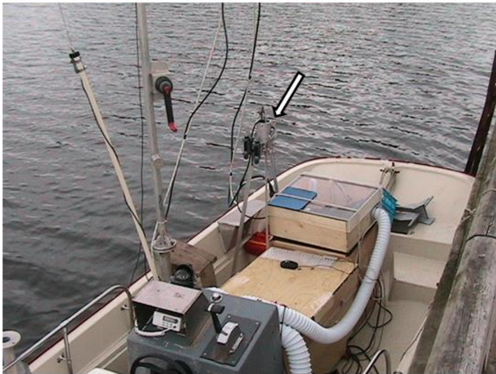
Figure 2: 2005 drop camera and sidescan arrangement on 15 foot Boston Whaler. Wooden boxes contain electronics, white tubing for ventilation. Top – arrow indicates sidescan hauled up for transport (note red tail); Bottom – arrow indicates drop camera frame on deck for transport.
