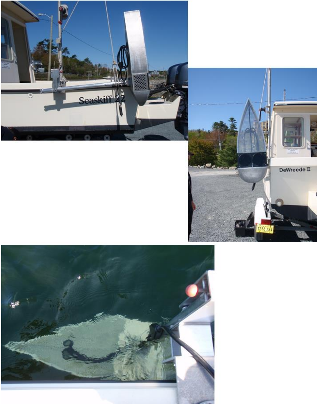
Figure 4: 2009-2011 new echosounder. Top – side view of transponder cage raised for transport; Middle – end view of raised cage; Bottom – cage immersed while on survey.
