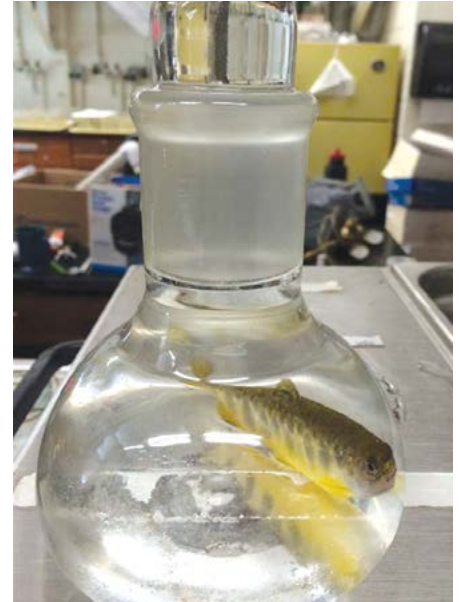
Juvenile Brook Charr in a respirometer used for measuring oxygen consumption. Photo: Kathleen O'Donnell (UNB)
