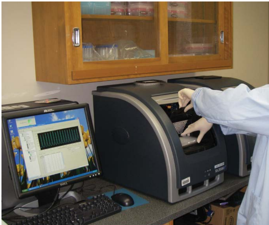
A quantitative polymerase chain reaction (PCR) machine, used to detect Viral Hemorrhagic Septicemia Virus (VHSV) genetic material. Photo: DFO
