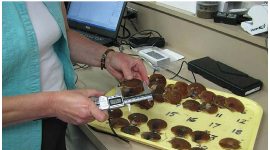
Measuring scallops using electronic calipers that register data directly in an Excel file. Photo: Leslie-Anne Davidson (DFO)
