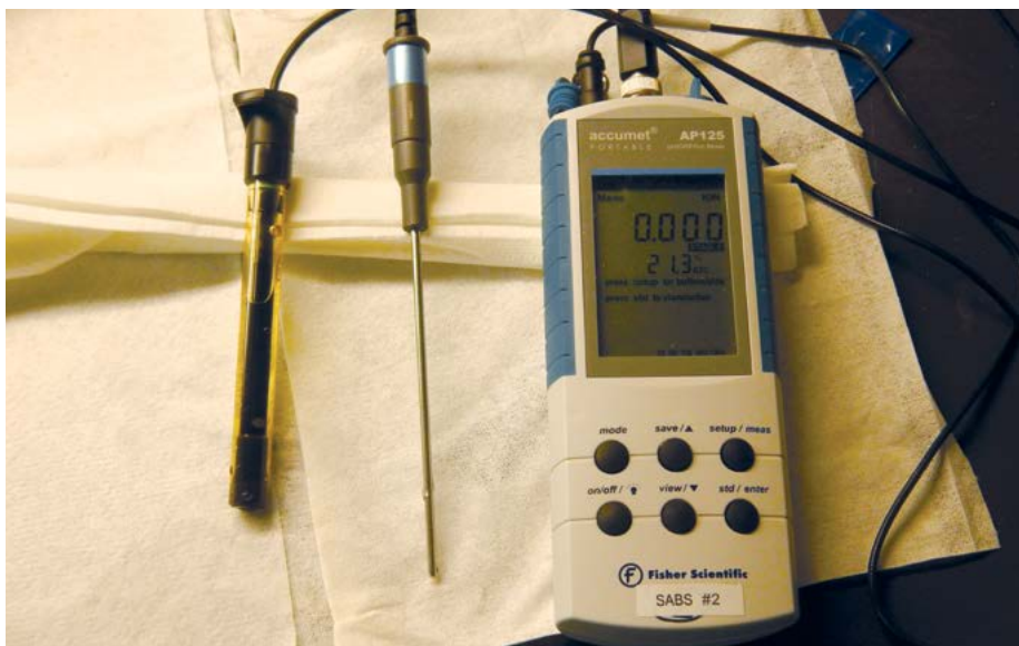
Photo shows sulfide probe, temperature probe, meter (left to right). Photo: Fred Page (DFO)
