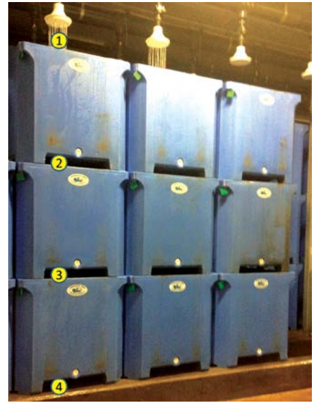
Stacked live mussel holding tanks. Water is introduced at the top, which then trickles down through the tanks to the bottom. Water sampling locations are indicated by the numbered yellow circles. Photo: Daniel Bourque (DFO)
