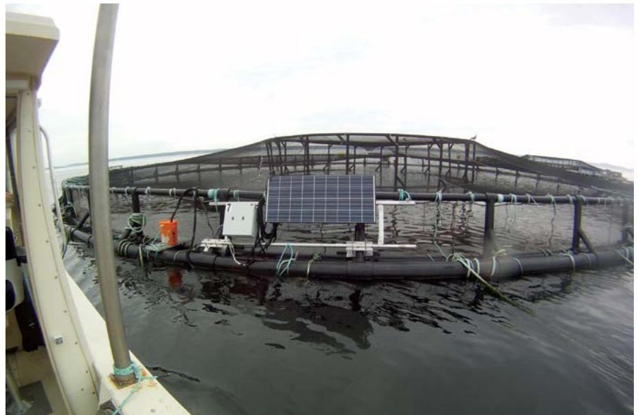
Solar powered sea lice light trap attached to a salmon cage in the Bay of Fundy. Photo: Nathaniel Feindel (DFO)
