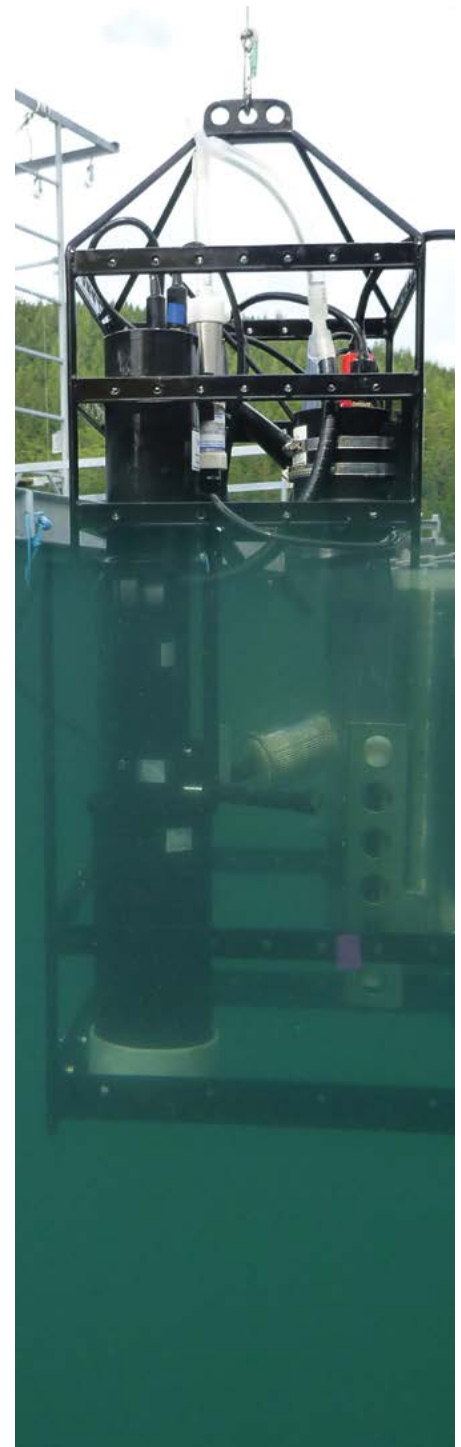
The bio-optical profiler being lowered into a Sablefish cage. Photo: Justin Del Bel Belluz (UVic)
