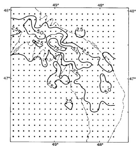
4. An example of a modelled output showing the number of calculated iceberg groundings per square kilometre (heavy contours) for a 1000-y period given the present mean iceberg flux and draught distribution onto the northeast Grand Banks. Centres of model cells are shown by the . . . symbol; bathymetry is in metres (the dashed contours).
