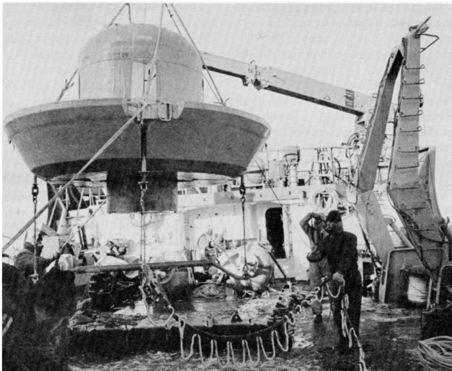
*Moorings about to be deployed from CSS Dawson in November 1985. These directional wave buoys are being used in the Canadian Atlantic Storm Project to measure wave height, and the direction of propagation of surface waters.*
