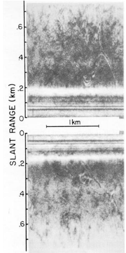
2. A sidescan sonograph of the Grand Banks seabed (at 133-m water depth) showing two populations of iceberg scour marks: a younger set of narrow continuous features superimposed on a degraded, discontinuous net work of older scour berms (ridges).
