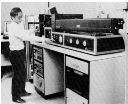
*Biologist William Li at the controls of a flow cytometer, an instrument that detects and measures fluorescent particles in sea water.*
