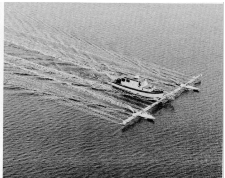
*The transportable "sweep" system provides total bathymetric survey coverage for charting of harbours.*
