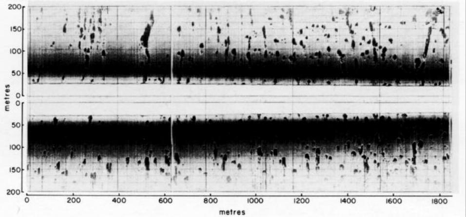
3. Sidescan sonogram across the Southeast Shoal on the Grand Banks showing a light-toned, sandy seabed with numerous dark patches interpreted as "shell beds". Some of the shell beds appear to be aligned in a bead-like fashion: this may result from control on their distribution by low relief bedforms.
