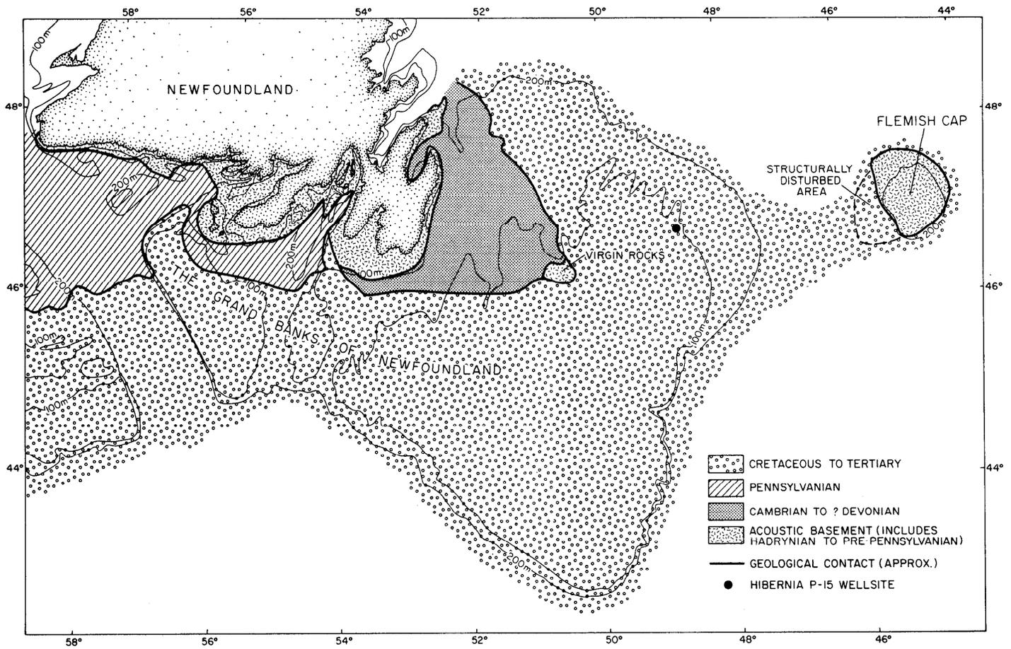
1. Generalized regional bedrock geology of the Grand Banks of Newfoundland and interpreted from seismic reflection profiles and analyses of electric rock core drill samples.
