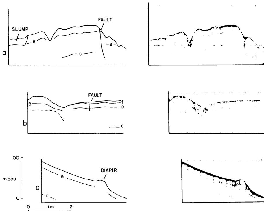
3. SeaMARC sidescan sonograph showing results of rotational slumping triggered by the 1929 Grand Banks earthquake.
