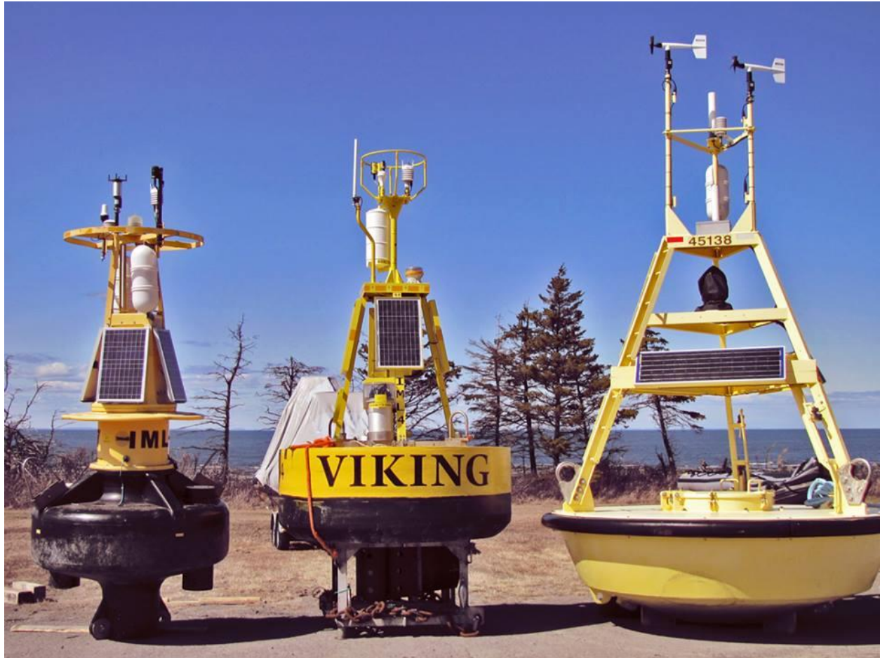
Figure A1.6 MLI and EC buoys. MOB of first generation (left), Viking MOB (4.5 m high and 2.1 m wide, center), EC meteorological buoy usually deployed at Mont-Louis station (right).
