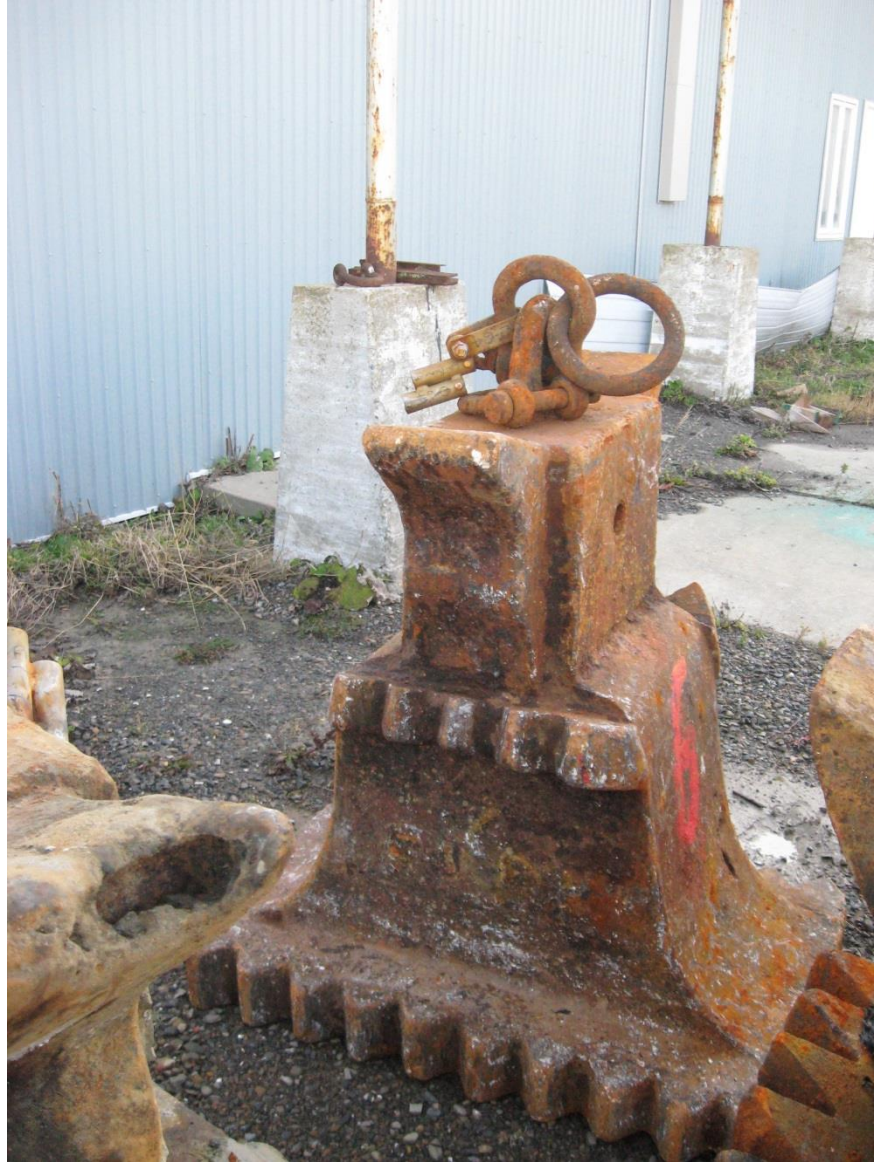
Figure A1.4 CCG buoy anchor. A thermograph support that can hold two instruments is bolted to the top. Here the anchor height (L) is 0.9 m.
