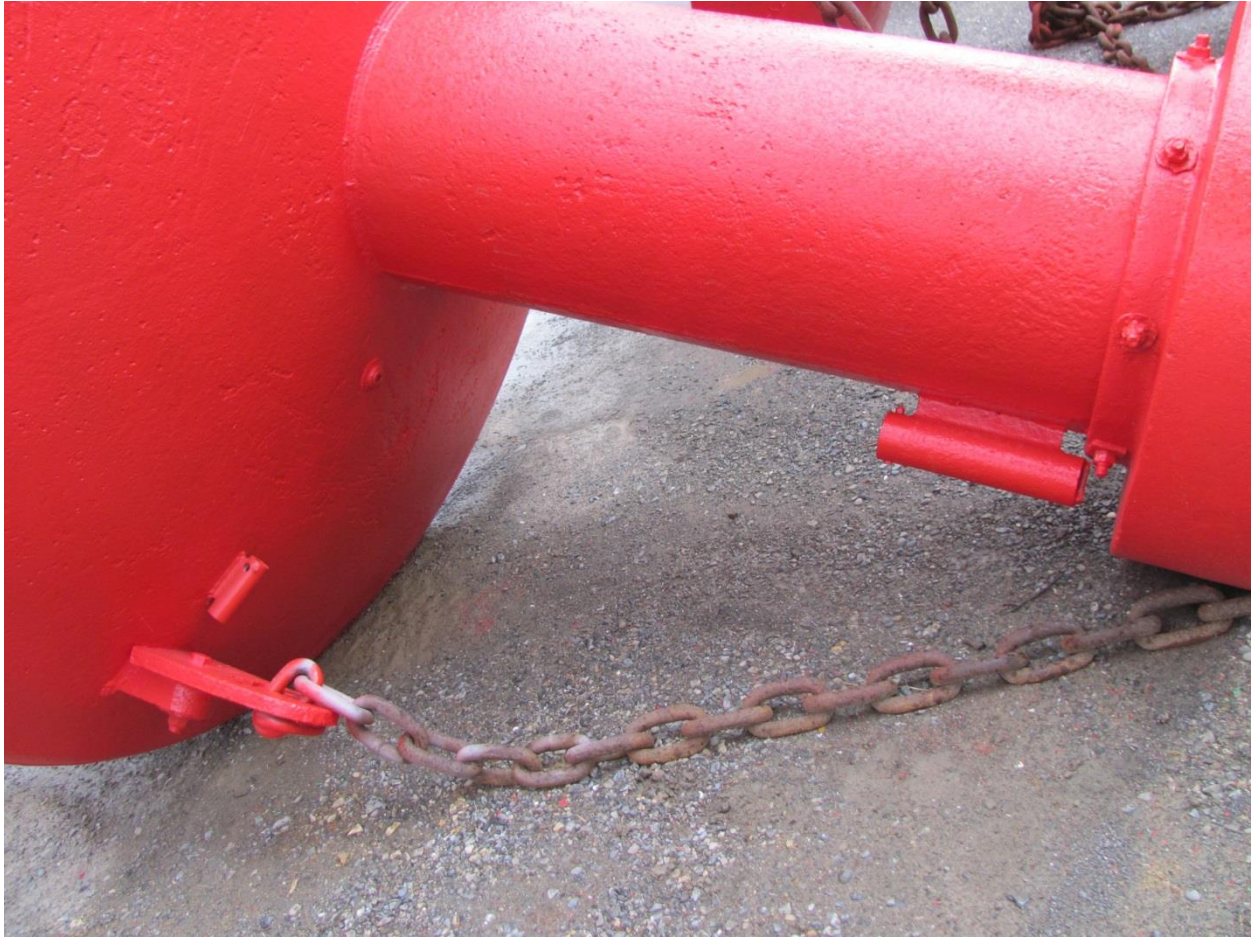
Figure A1.3 Thermograph support bracket on CCG buoy. The support bracket at the left is welded under the hull behind the mooring chain buoy bracket, for measurements at 0.5 m depth. The other larger support shown at the right is welded on the buoy foot at 2 m depth.
