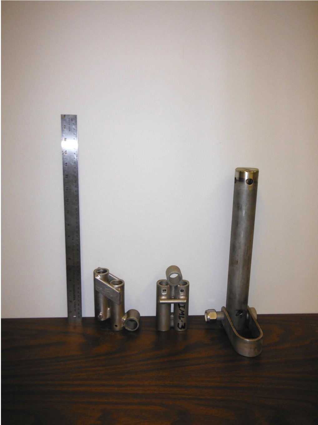
Figure A1.2 Instrument support brackets for buoy anchors. From left to right: 45.7 cm long ruler for scale, support that can hold two instruments, a variant of the first support model that can also hold two instruments, and the latest support specially made for the SBE-56.
