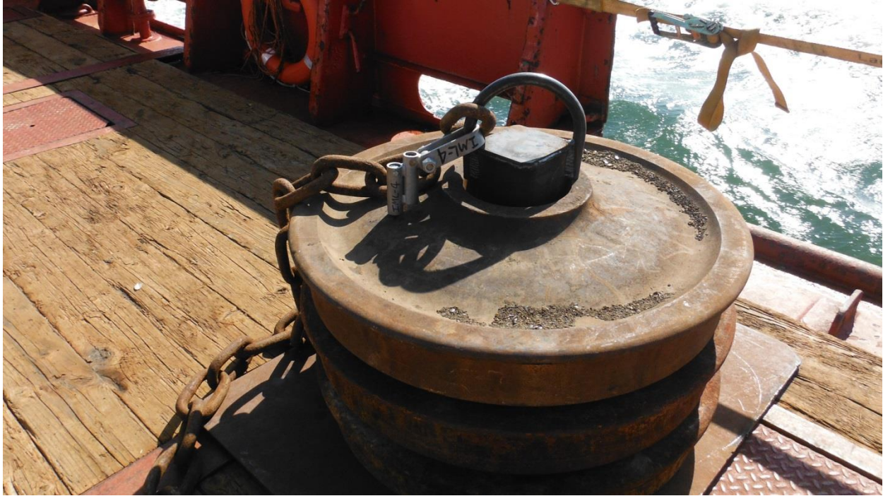
Figure A1.5 MLI buoy anchor. Three train wheels attached to a metal plate are used to anchor buoys like the Viking MOB. The thermograph support bracket is bolted to the ring on top of the anchor. The anchor height is 0.75 m. Anchors with only one or two train wheels are used for lighter buoys.
