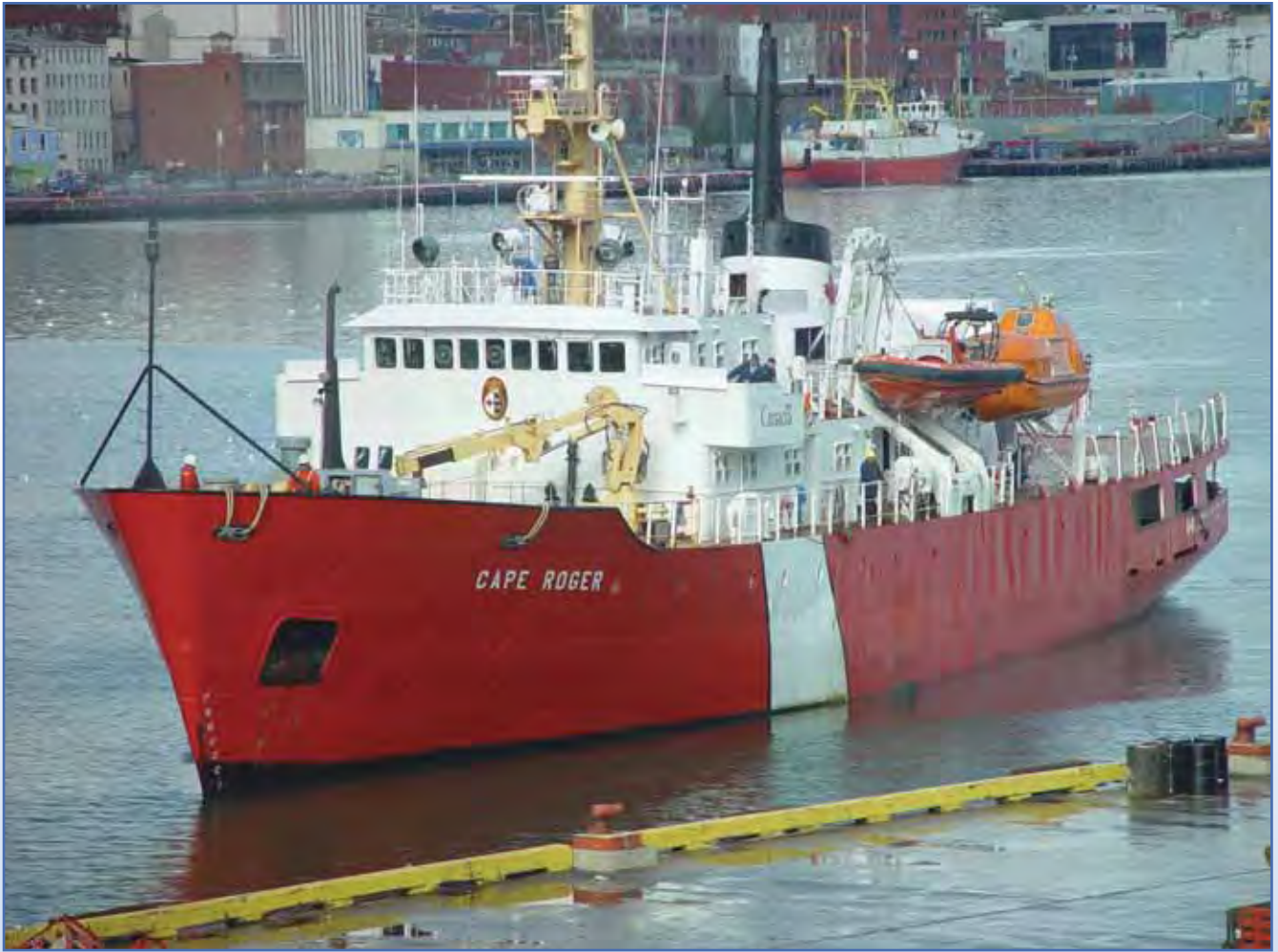
CCGS Cape Roger , an Offshore Patrol Vessel, showing the effects of sustained at-sea operations during heavy weather. Photo: NL Region
