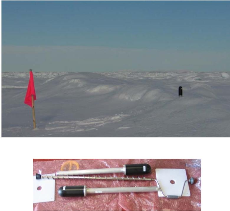
Fig. 38 Iridium beacon deployed on a MYI floe in Kennedy Channel (above) and beacons with 2" ice auger used to deploy the beacons (below).
