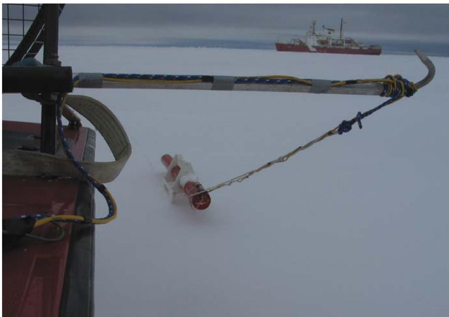
Fig. 16 EM sled being towed by the “Skippy Boat” over a FYI floe north of Peel Sound on September 1 on a typical overcast day when surface topography is obscured.
