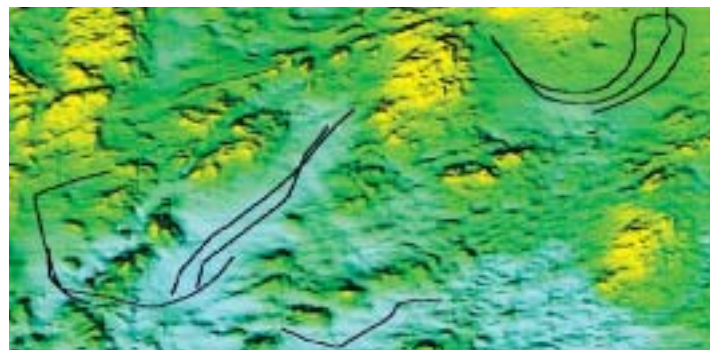
Figure 1. Using a three-dimensional bathymetric chart of Browns Bank, a captain is able to alter course during tows to avoid rough bottom and obstacles that could damage the gear.
