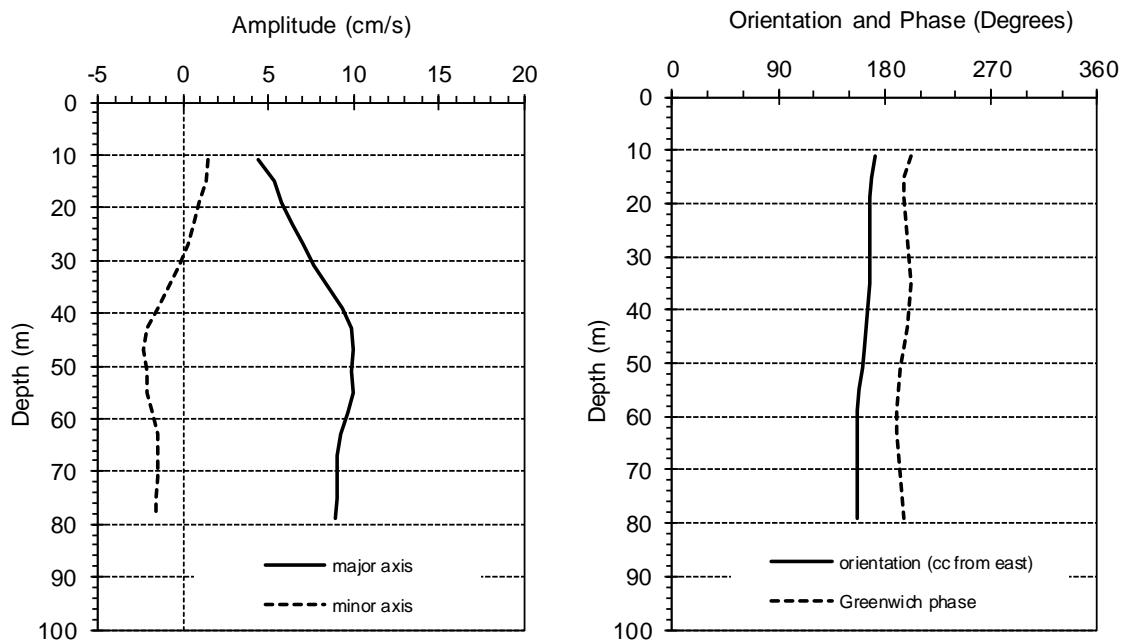
**Figure 35: O1 Tidal Constituent, South Side of Barrow Strait**
