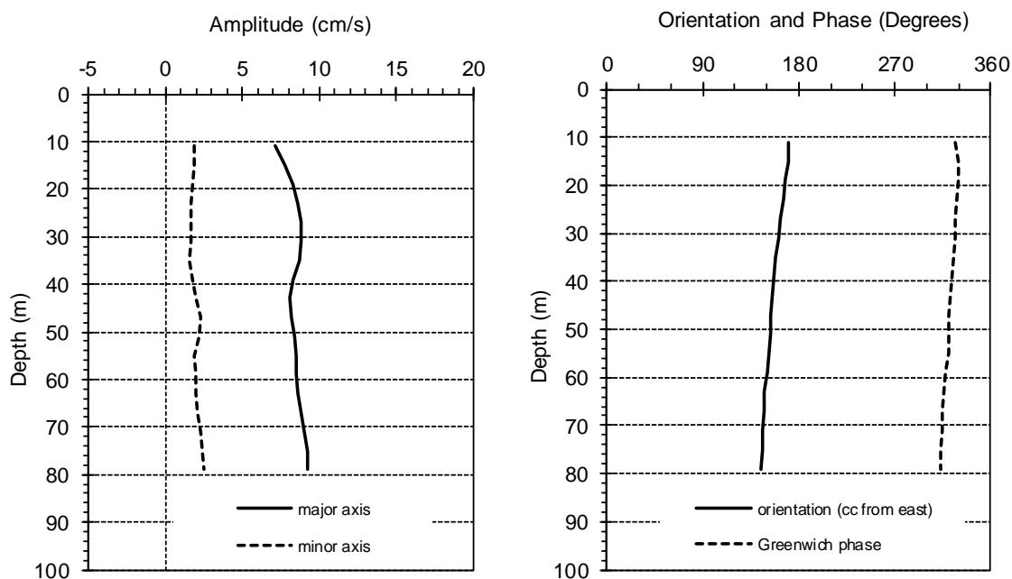
**Figure 34: M2 Tidal Constituent, South Side of Barrow Strait**
