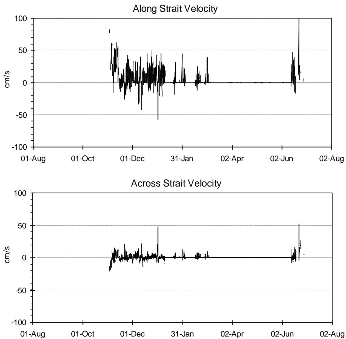
**Figure 49: Ice velocity data, South-Central Barrow Strait
