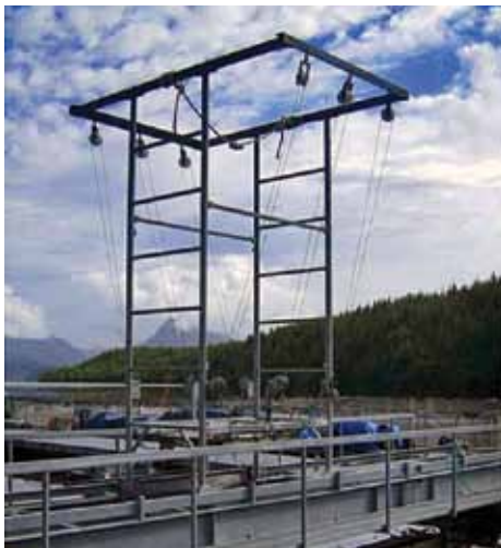
The SEAt tram shellfish system and hoists developed at the Kyuquot SEAfoods Ltd. IMTA site. Photo: Eric Hovenaars (UVic)
