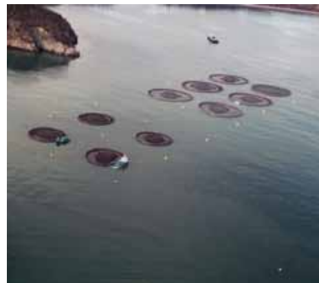
Salmon aquaculture farm in the Bay of Fundy, NB. Polar circle cages are arranged over a square sub-surface grid configuration. Photo: Cooke Aquaculture Inc.
