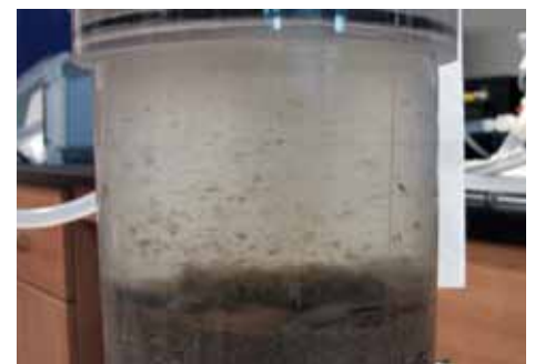
In-laboratory erosion measurements of mussel aquaculture waste using a Gust microcosm erosion chamber and a sandy seabed. Applied bed shear stress of 0.08 Pa is strong enough to mobilize the waste material and re-suspend large aggregates. Photo: Particle Dynamics Lab, BIO (DFO)
