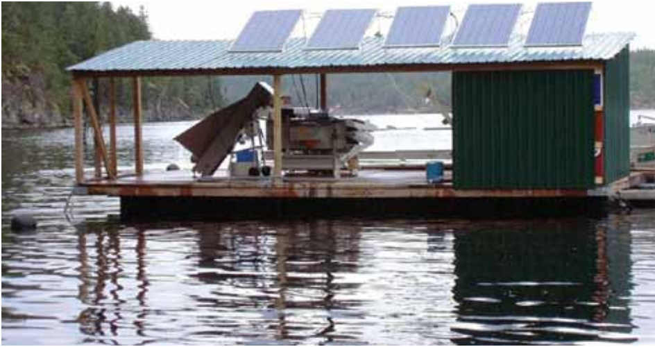
Mobile floating seed sorter and handling system. Photo: Yves Perreault (Little Wing Oysters Ltd.)
