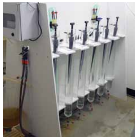
Experimental flow-through system used at IFREMER. Photo: Marine Holbacg (IFREMER)
