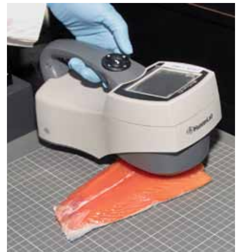
Colourimeter used to measure the colour in salmon fillets. Photo: Sébastien Plante (UMCS)
