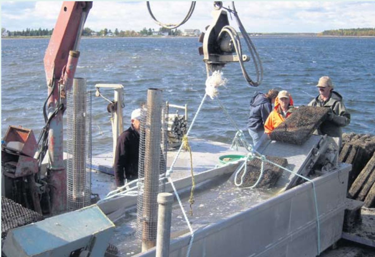
Hot water bath for control of biofouling organisms. Conveyor belt drives Vexar® bags in hot water.
