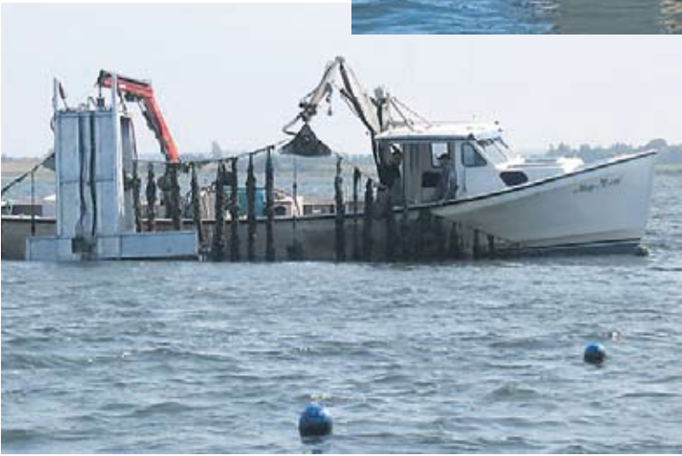
Above: Lime treatment system used to treat the clubbed tunicate in Malpeque Bay, recovers the lime in the horizontal part of the mechanism for re-use. This system belongs to Martin MacDonald.
