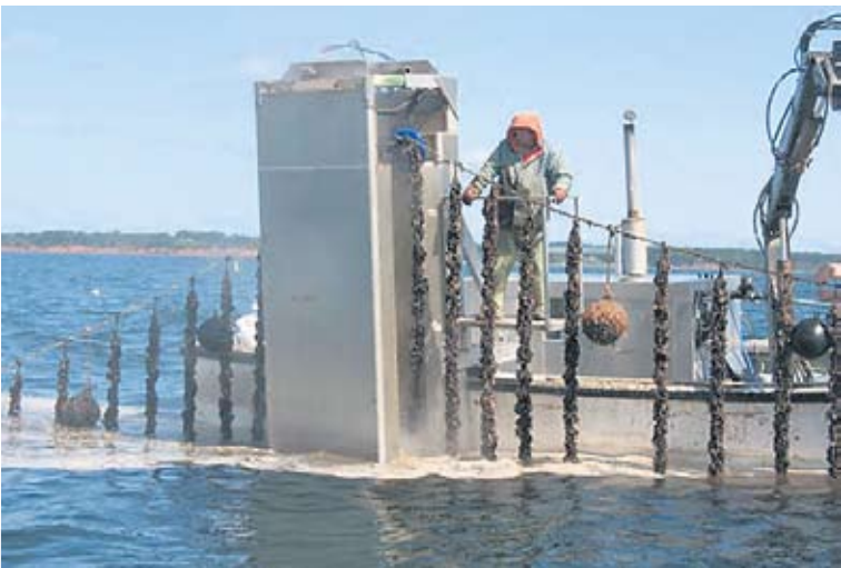
Above: Lime treatment system used to treat the clubbed tunicate in Malpeque Bay, recovers the lime in the horizontal part of the mechanism for re-use. This system belongs to Martin MacDonald.
