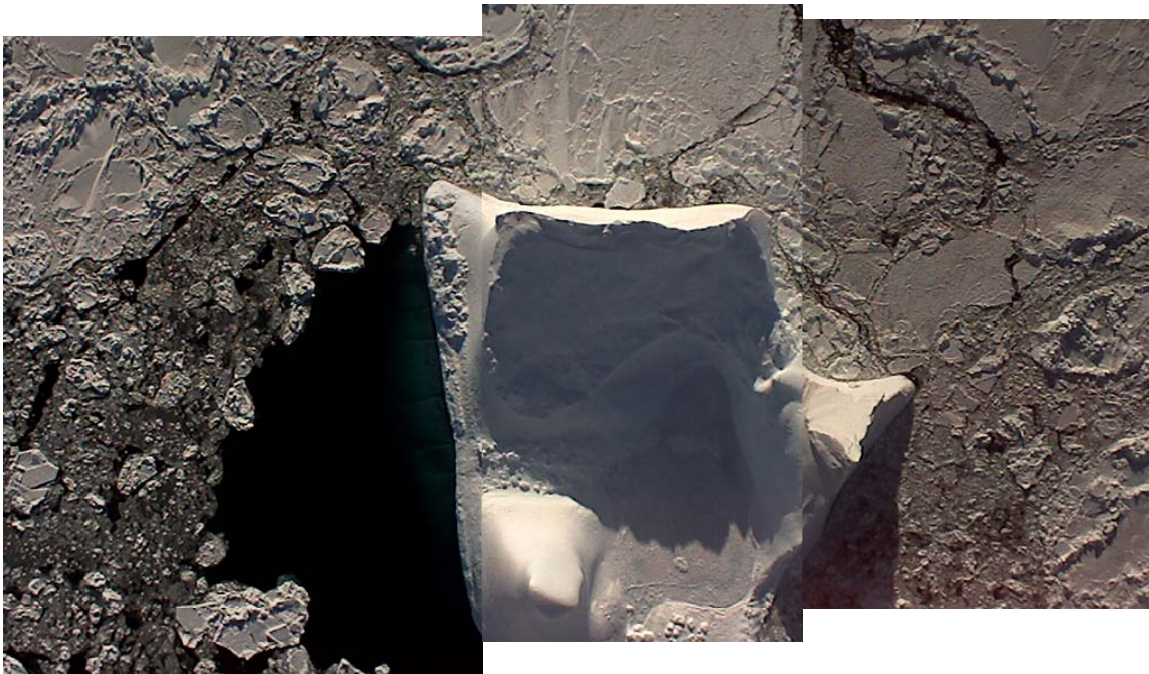
Fig. 24 Pinnacle iceberg mosaic from Video frames taken at a height at 120m providing frame widths of 132m (March 19). Pinnacle iceberg about 100mx100m. ARGOS ice beacon 12995 deployed on berg (Video frame 28393).
