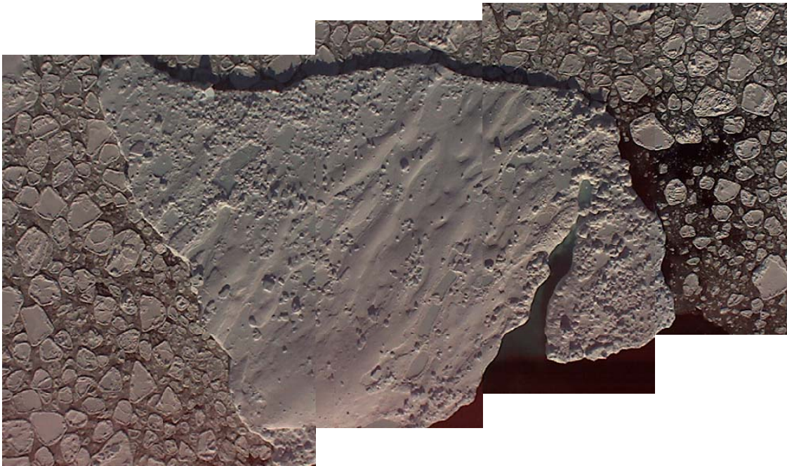
Fig. 27 Mosaic of small iceberg made of video frames taken at 133m height providing frame widths of 145m. Iceberg about 145mx160m; freeboard by Laser ~4.5m. Iridium beacon 2484860 (video frame 31610).
