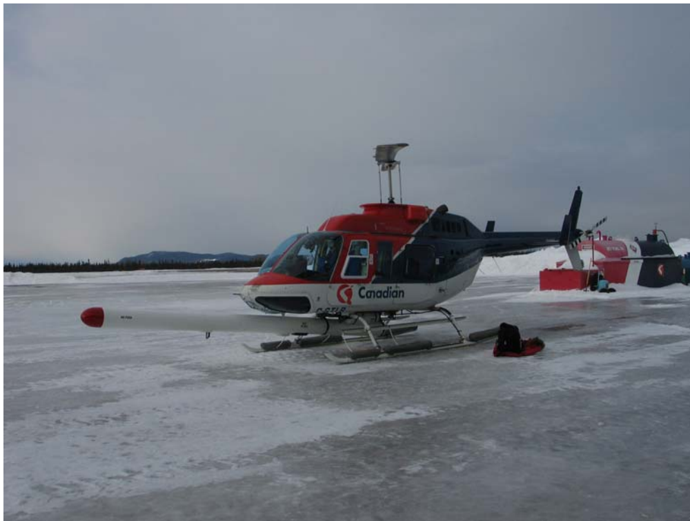
Fig. 1 Canadian Helicopters Ltd. 206L helicopter with the fix-mounted sensor equipment (March 2011). The EM sensor is located in the outer section and the GPR and Video-Laser are located in the middle section of the “cigar” shaped mount.
