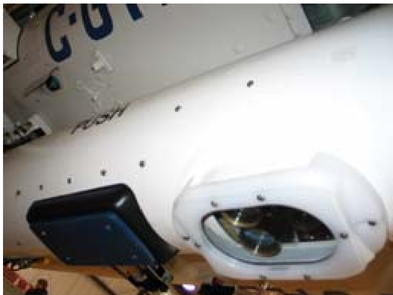
Fig. 2 Sensors and Software Noggin 1000-NIC GPR System (left) protruding from middle section of the mounting tube along with laser/video camera (right).
