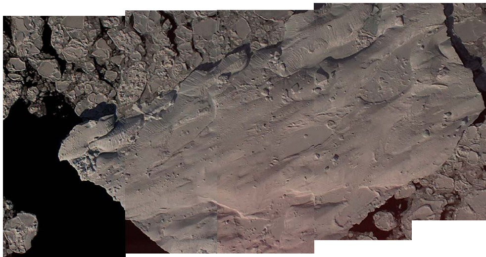
Fig. 22 Video mosaic of tabular iceberg or ice island fragment; video data taken from 122m height providing frame widths of 135m. The iceberg is about 100mx200m, has a freeboard estimated with laser of 5.3m. Argos beacon 12997 was deployed on iceberg on March 19, Video frame 34520.
