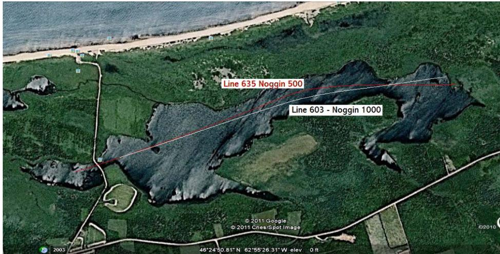
Figure 1.3 - Google Earth image locating the Noggin 500 and Noggin 1000 GPR profiles flown over a small Lake in Prince Edward Island.
