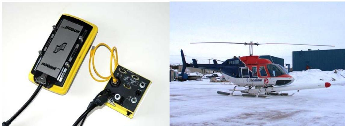
Figure 1.1 Sensors and Software Noggin 1000 GPR and NIC control unit (left) and the mounting boom under the Bell 206L Helicopter (right).
