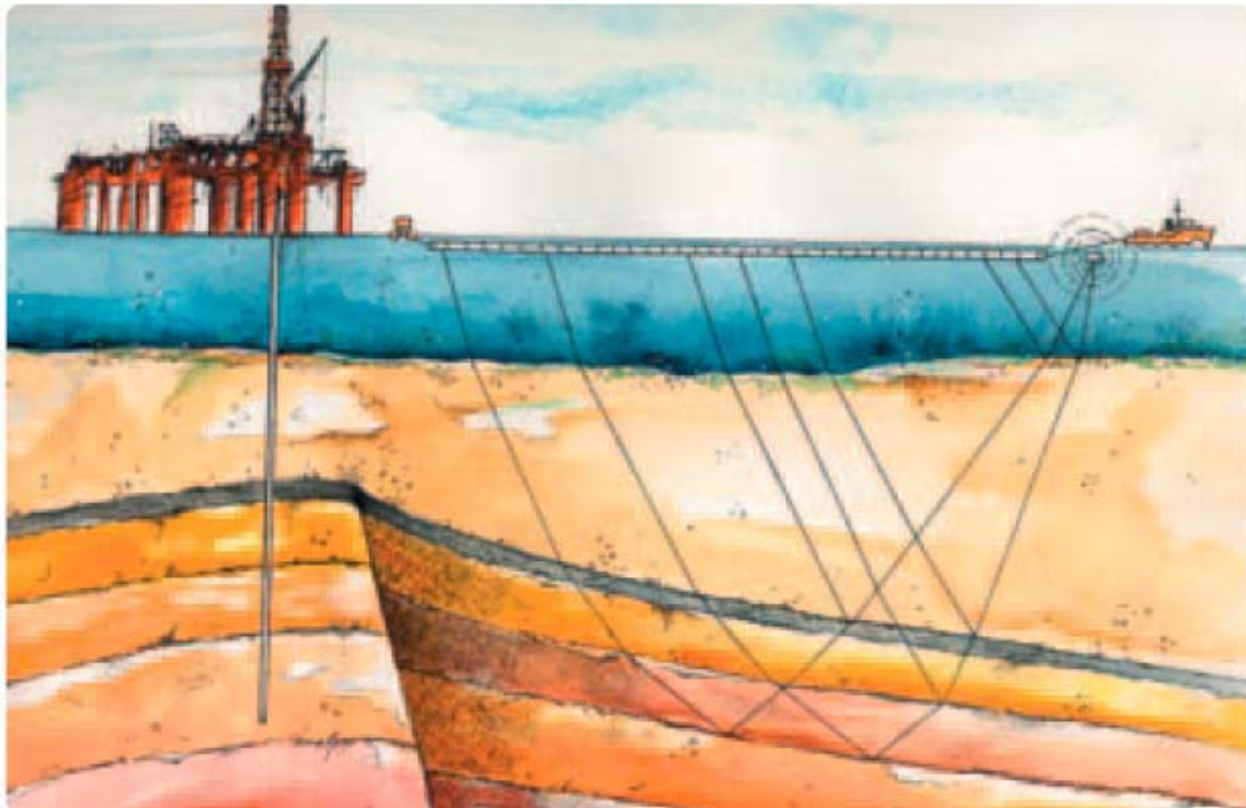
Figure 1. A signal source and one or several cables are towed behind a seismic vessel. The sound signals from the air gun are sent into the seabed and reflected by the various stratigraphic layers before being registered by the hydrophones inside the cables (OLF, 2004).
