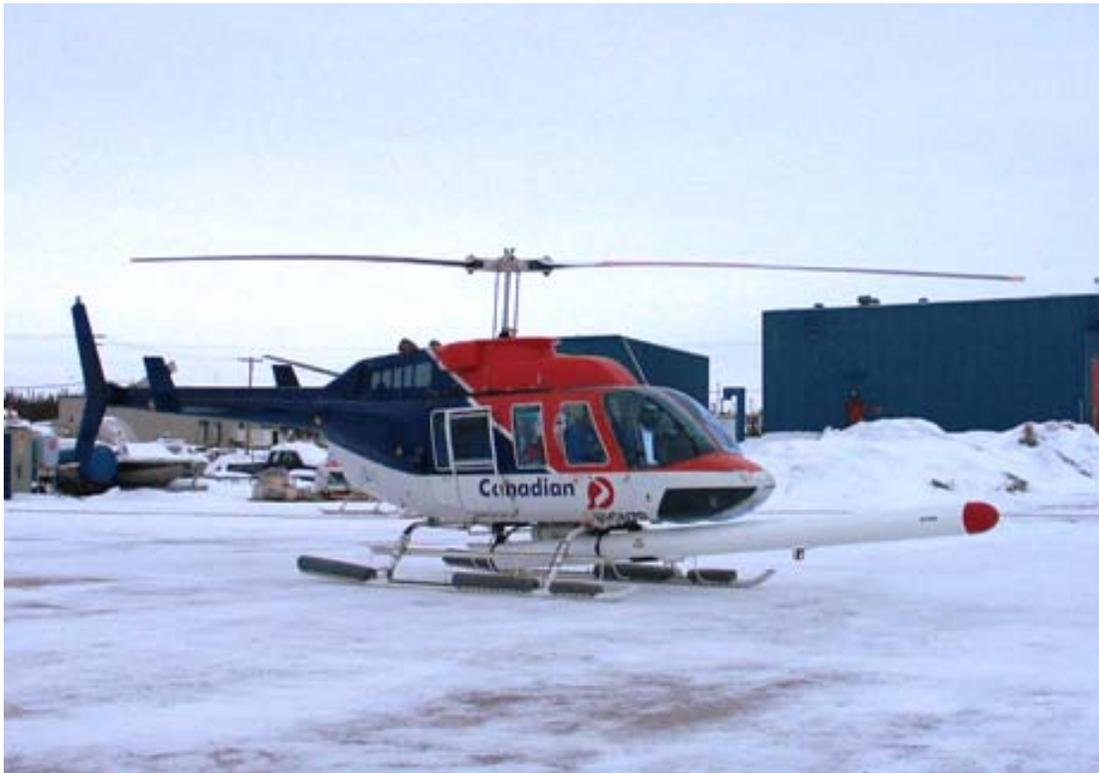
Fig. 1 Canadian Helicopter 206L showing the fix-mounted sensor equipment. The EM sensor is located in the outer section and the GPR and Video-Laser are located in the middle section of the “cigar” shaped mount.
