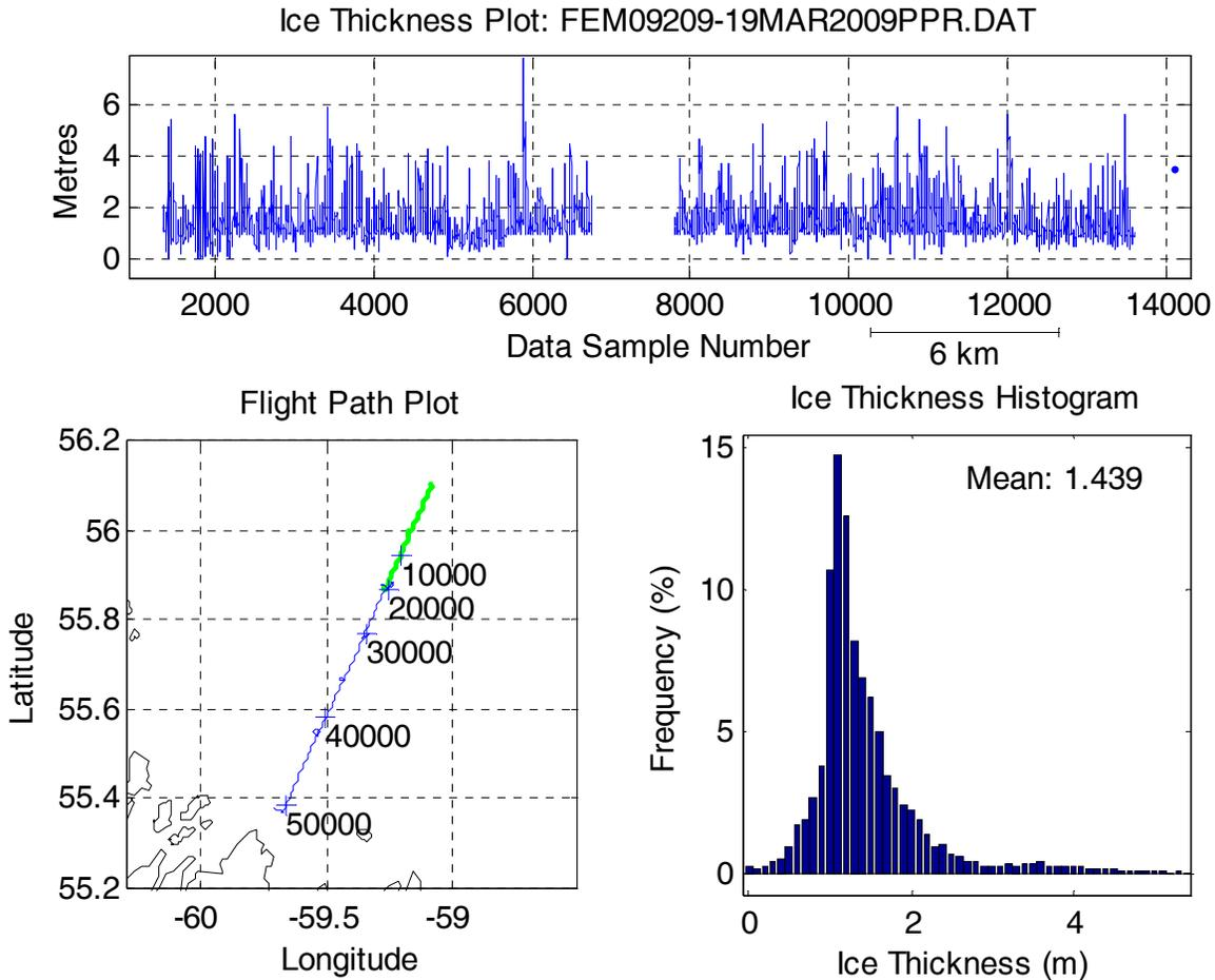
Fig. 8 Offshore sub-section (~30km) of the ice thickness data from the “middle” survey line. The green line in the map shows where the ice thickness profile data plotted and used to derive the histogram were collected.
