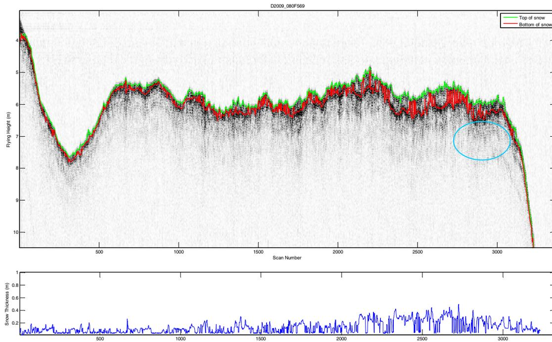
Fig. 45 GPR line plot and snow thickness of First Site 21-1 GPR 570 line flown South to North.
