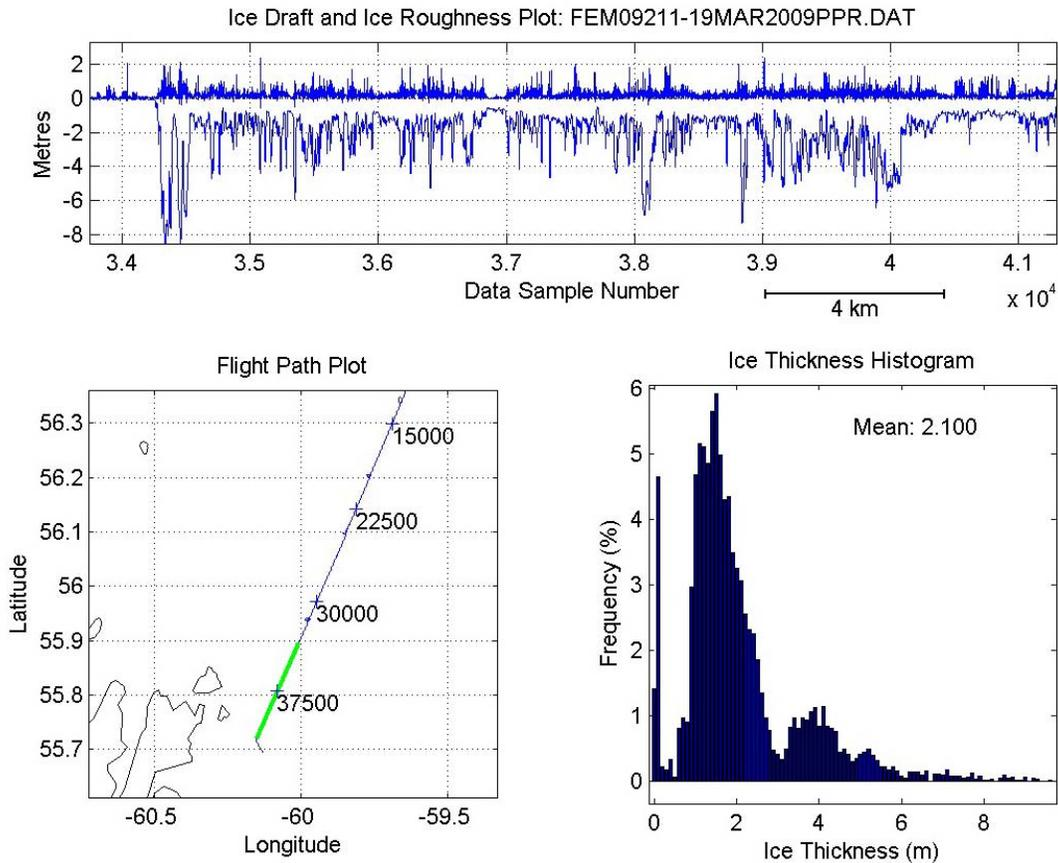
Fig. 30 Land-fast ice section plot off Hopedale, March 19. Thin ice offshore of the shear ridge located at sample number  $3.45 \times 10^4$  with the left side representing the offshore end and right the inshore end of the profile plot.
