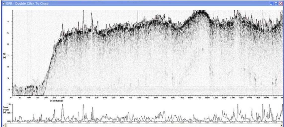
Fig. 21 Start of GPR line #535 showing ~2km of GPR-Laser profile and resulting snow thickness profile. Left side is offshore and right side inshore.
