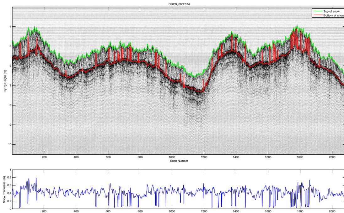
Fig. 46 GPR line plot and snow thickness of second Site 21-2 GPR 574 line flown South to North.
