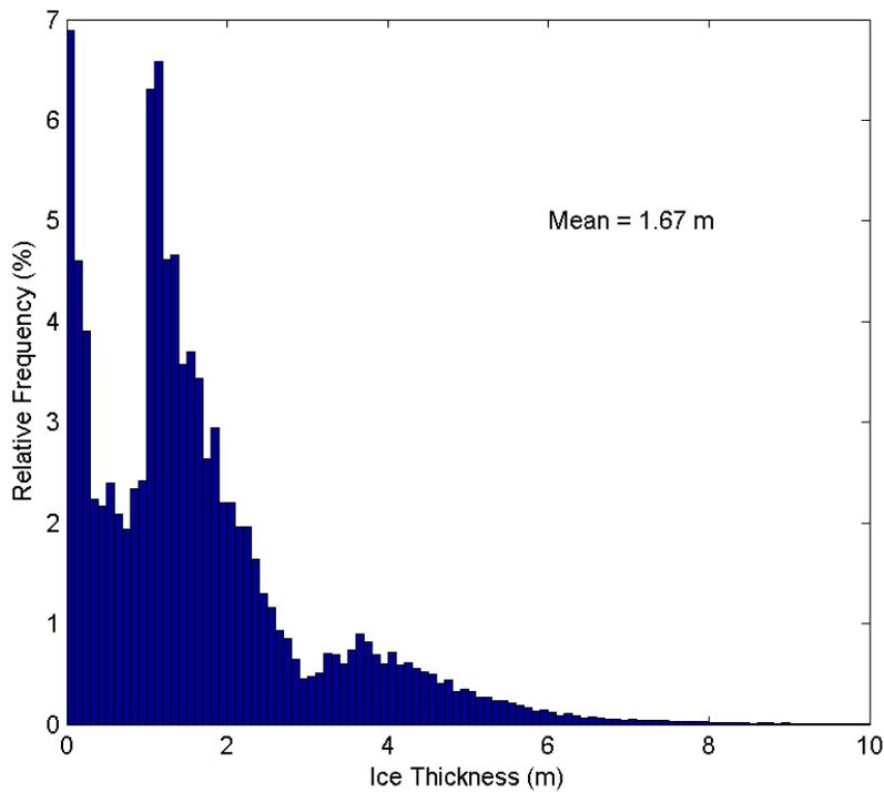
Fig. 19 Combined ice thickness histogram of the ice thickness profiles collected off the Labrador coast during March 2009. (Total profile distance of 550km)
