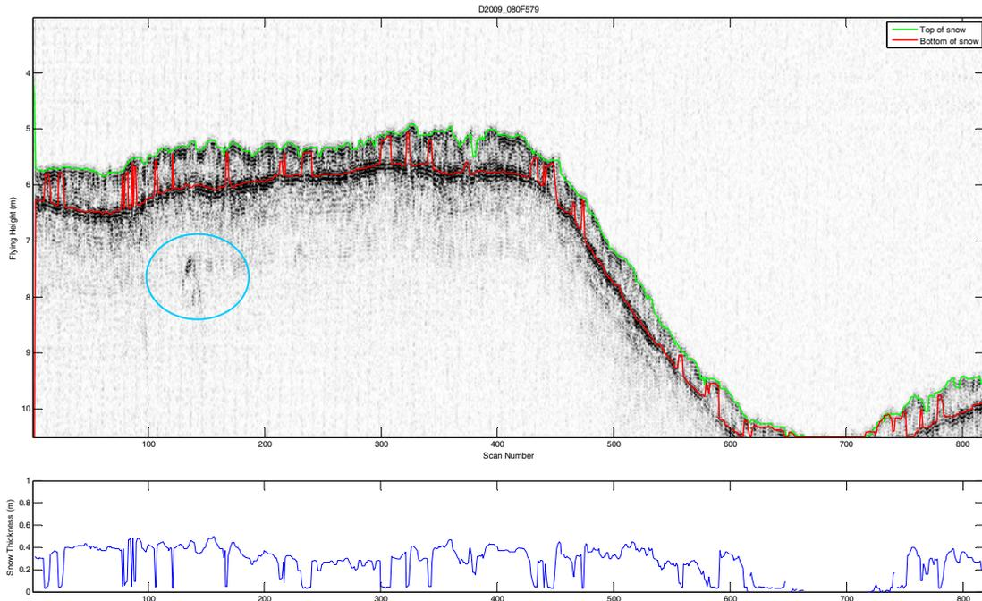
Fig. A5 GPR line plot and snow thickness of third Site 21-3 GPR 579 line flown East to West. This site (Fig. A5 and A6) has a thick snow layer like Site 21-2.
