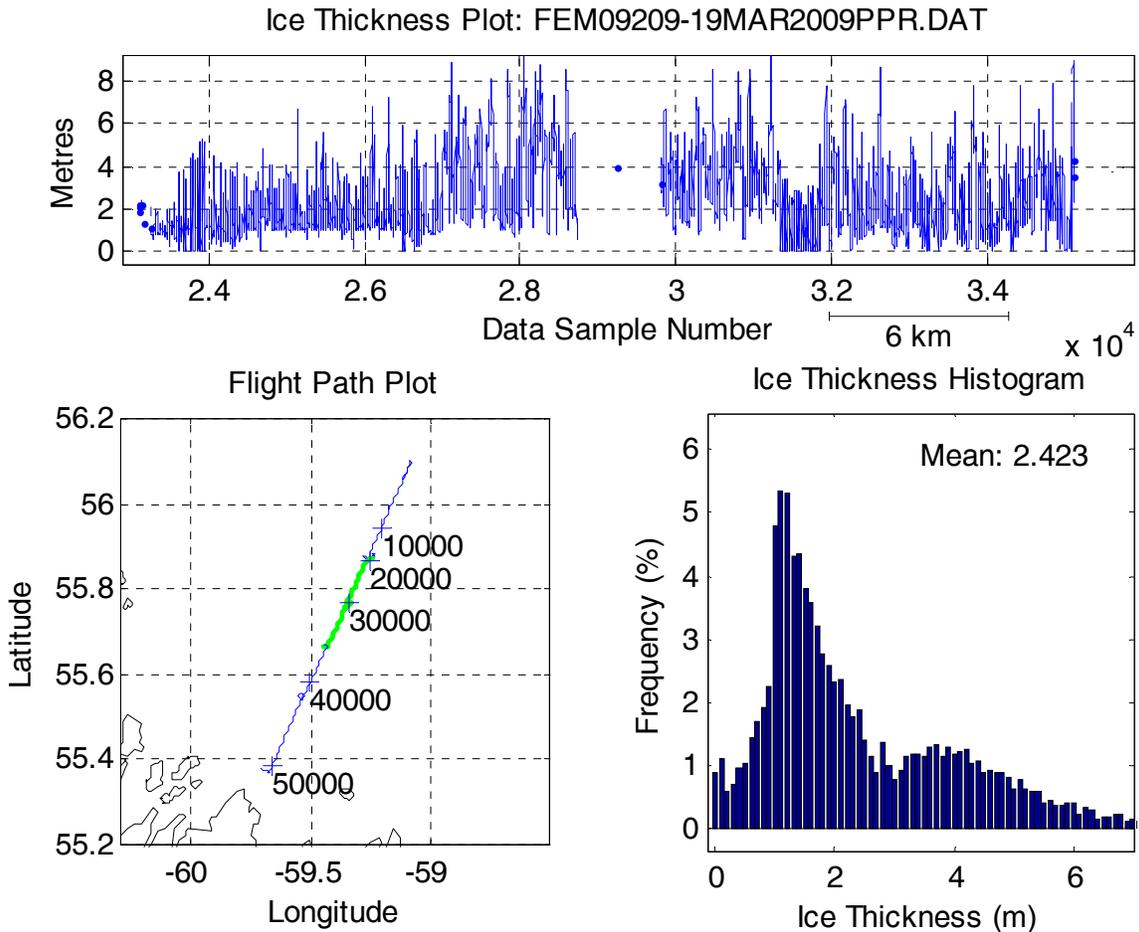
Fig. 11 Middle sub-section (~28km) of the ice thickness data from the “middle” survey line (left is offshore and right inshore). The green line in the map shows where the ice thickness profile data plotted and used to derive the histogram were collected.
