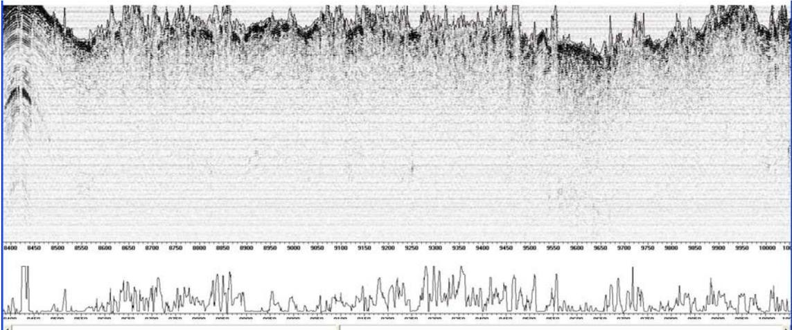
Fig. 29 Middle of GPR line #539 showing ~2km of GPR-Laser profile and resulting snow thickness profile. Section is about 7km from the land-fast ice edge with the offshore side on the left and the inshore side on the right.
