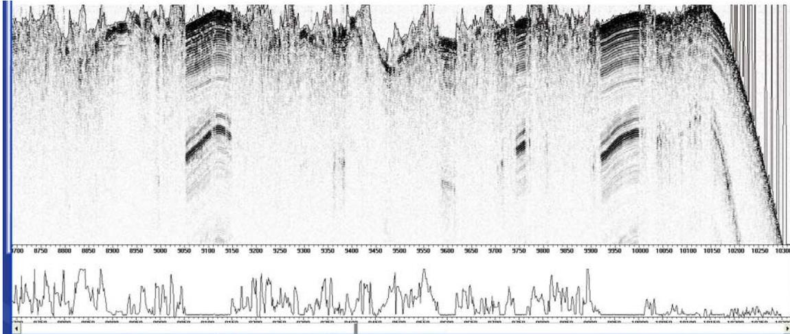
Fig. 27 Middle of GPR line #538 showing ~2km of GPR-Laser profile and resulting snow thickness profile. Section is about 18km from the land-fast ice edge, with the offshore side on the left and the inshore side on the right.
