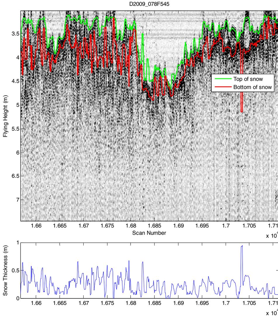
Fig. 31 GPR line section plot of F545 at transition from rough land-fast ice to mainly smooth land-fast ice. The EM plot for the same area (Fig. 30) indicated a change from thick to thinner land-fast ice.
