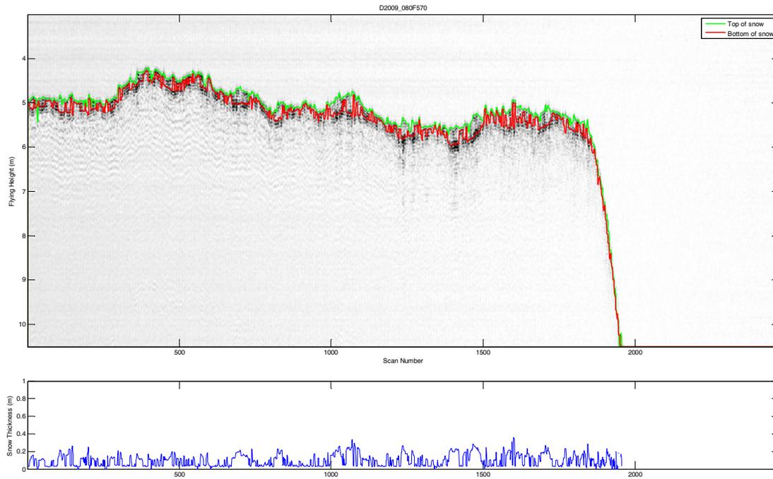
Fig. A2 GPR line plot and snow thickness of First Site 21-1 GPR 569 line flown West to East. This site (Fig. A1 and A2) has less snow than the other two sites within Lake Melville.
