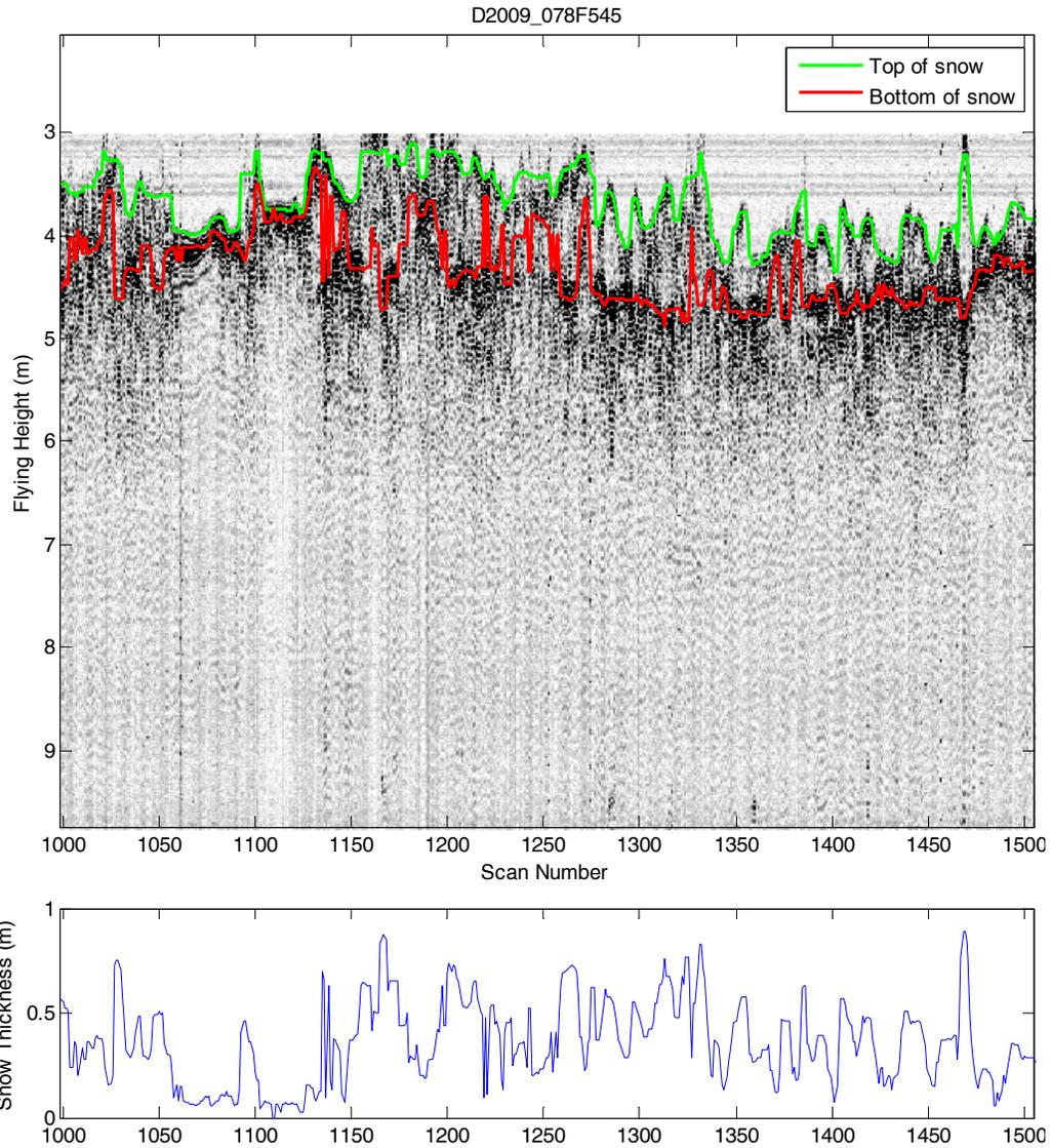
Fig. 32 GPR snow thickness profile (~0.5km) of the rough/thick land-fast ice off Hopedale at about 1.0 to 1.5km inshore of the shear ridge (start of GPR line section 545 Fig. 20).
