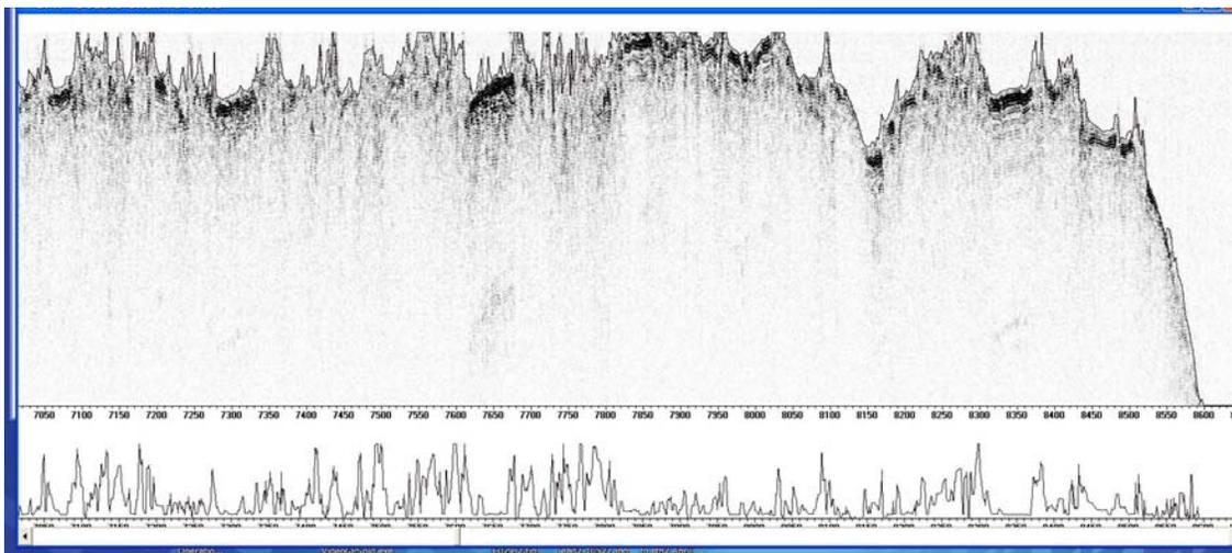
Fig. 24 Middle of GPR line #537 showing ~2km of GPR-Laser profile and resulting snow thickness profile Left side is offshore and right side inshore.
