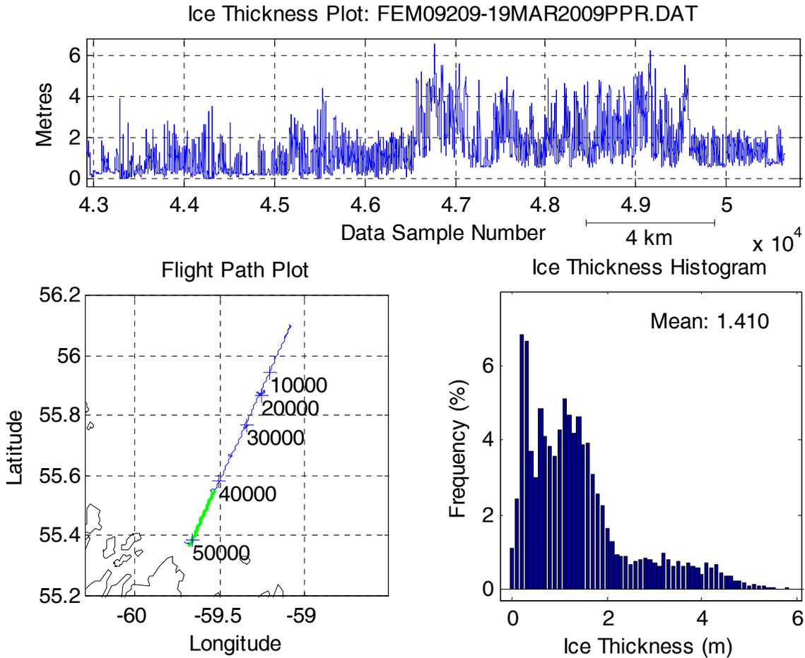
Fig. 14 Inshore sub-section (~24km) of the ice thickness data from the “middle” survey line. The green line in the map shows where the ice thickness profile data plotted and used to derive the histogram were collected. The thin ice area with frost flowers is on the left and the land-fast ice is on the right starting at sample #  $4.65 \times 10^4$ .
