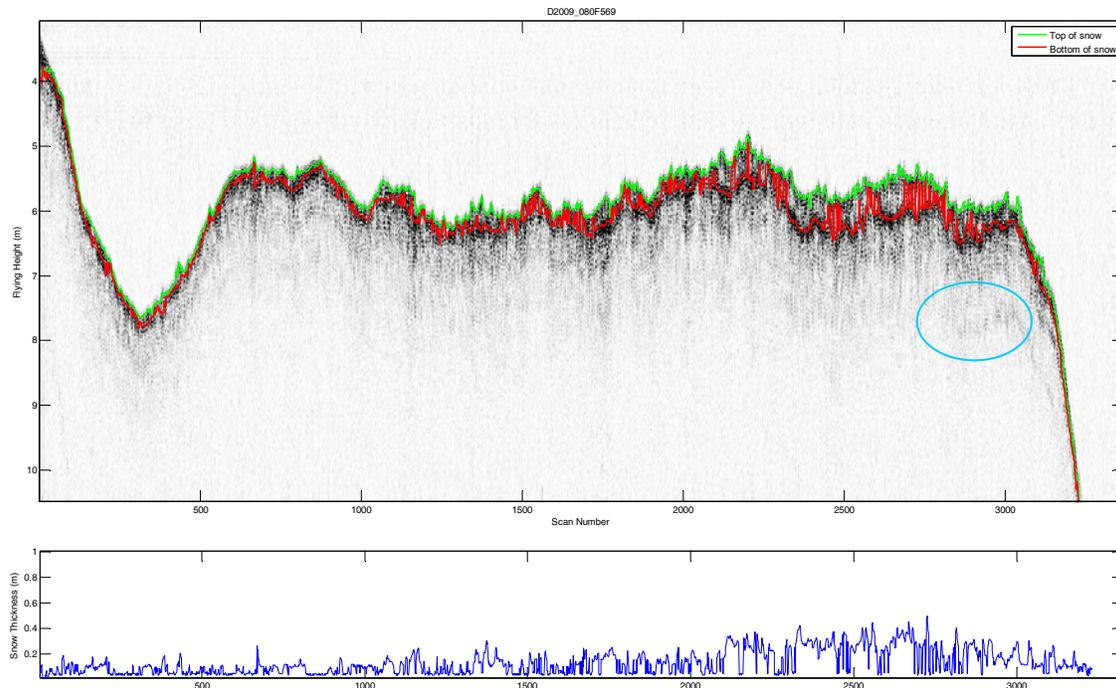
Fig. A1 GPR line plot and snow thickness of First Site 21-1 GPR 570 line flown South to North. This site (Fig. A1 and A2) has less snow than the other two sites within Lake Melville.
