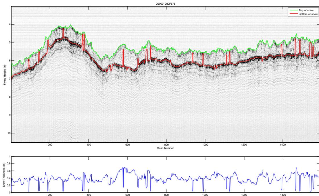
Fig. A4 GPR line plot and snow thickness of Second Site 21-2 GPR 575 line flown East to West. This site (Fig. A3 and A4) has more snow than site 21-1.
