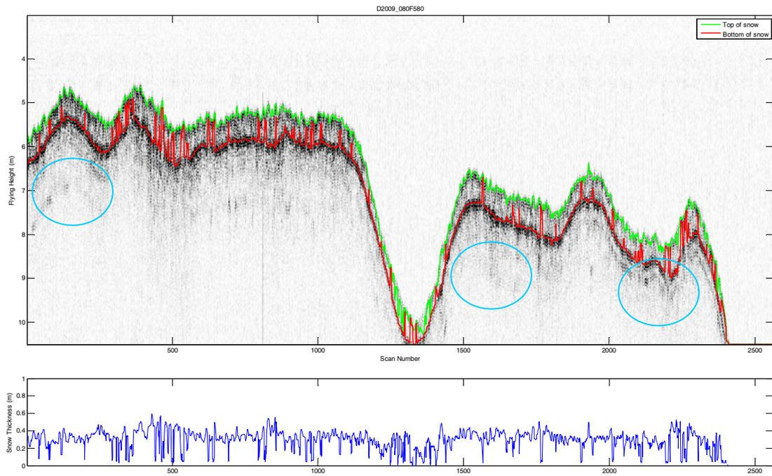
Fig. A6 GPR line plot and snow thickness of third Site 21-3 GPR 580 line flown South to North. This site (Fig. A5 and A6) has a thick snow layer like Site 21-2.
