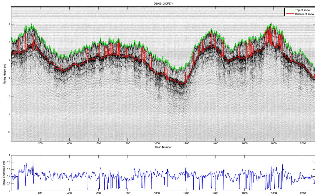
Fig. A3 GPR line plot and snow thickness of second Site 21-2 GPR 574 line flown South to North. This site (Fig. A3 and A4) has more snow than site 21-1.
