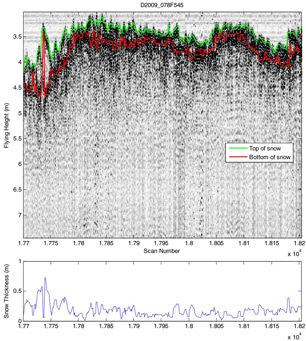
Fig. 33 GPR snow thickness profile (~0.5km) of the smooth/thin land-fast ice off Hopedale at about 18km inshore of the shear ridge (end of GPR line section 545 Fig. 20).
