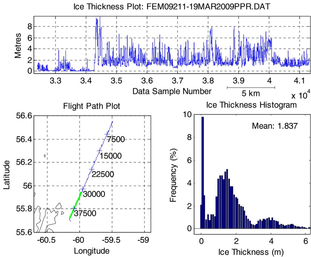
Fig. 16 Inshore sub-section (green line ~32km on map) of the ice thickness data of the Hopedale line, showing shear ridge and land-fast ice (left is offshore and right inshore).
