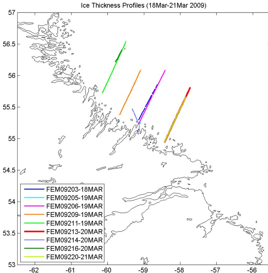
Fig. 3 Survey lines off the Labrador coast along which EM ice thickness, Laser ice roughness and experimental GPR snow thickness data were collected. Line numbers represent the EM file numbers and dates when the data were collected. The four line locations are Hopedale (north), “middle”, Makkovik, and mooring line (south).
