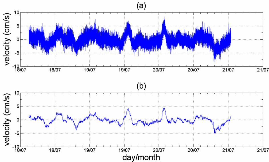
Figure 3. Time series of (a) unfiltered velocity profiles taken at site 2 (coral area) from transducer beam 1, profile bin 1 (1 meter above the instrument) and (b) same time series after filtering with Butterworth low pass filter cutoff frequency of  $3 \times 10^{-3} \text{ Hz}$ .
