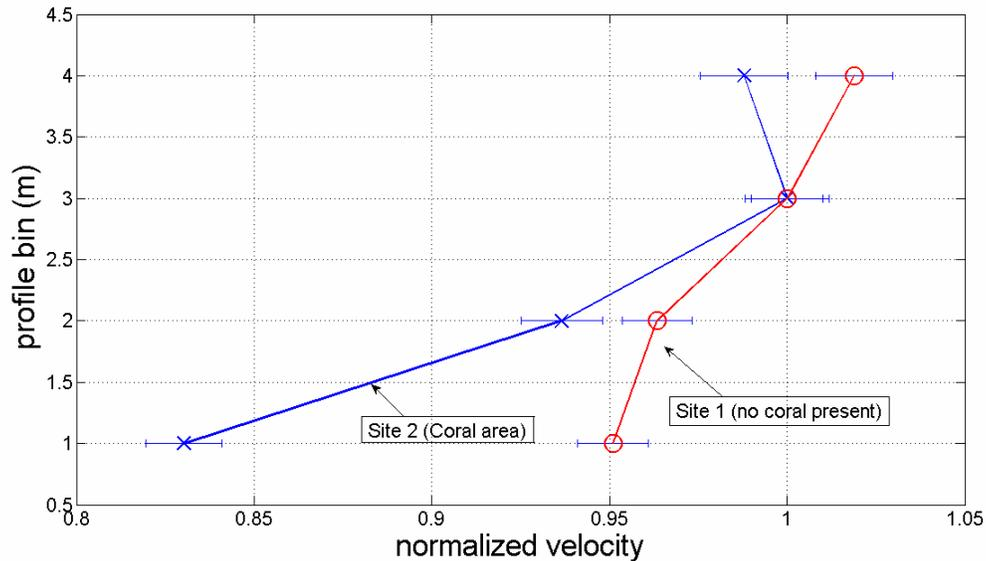
Figure 5. Mean velocity profile comparison for the coral area (Site 2, 'X') and non-coral area (Site 1, 'O'). The x axis is the velocity normalized by the bin 3 velocity. The y axis is the height above the profiler in meters.
