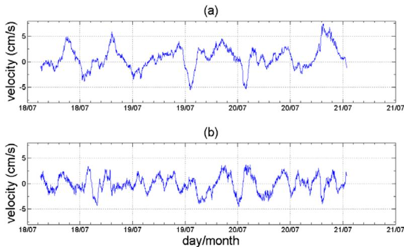
Figure 4. Time series of (a) East velocity for site 2 (coral area), the magnitude of observed velocities was between 0-10 cm/s, which is low compared with currents observed in other coral habitat (10-30 cm/s), evidence of tidal signals and non-linear processes is also identified, and (b) North velocity time series for site 2 (coral area).
