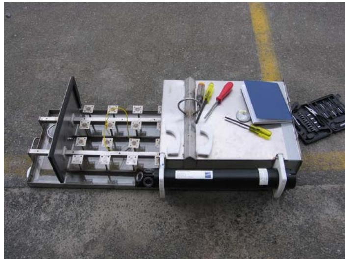
Figure 1. Settling plate with Nortek Aquadopp 2 mHz doppler profiler during initial fitting of the profiler at Oceans Science Center, Logy Bay. The settling plate is approximately 121 cm (48 inches) long, 45 cm (18 inches) wide, and 30 cm (12 inches) high.
