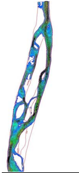
Fig. 1. Example of highly complex depth and velocity solutions within the Athabasca River derived from application of a two-dimensional hydrodynamic model.
