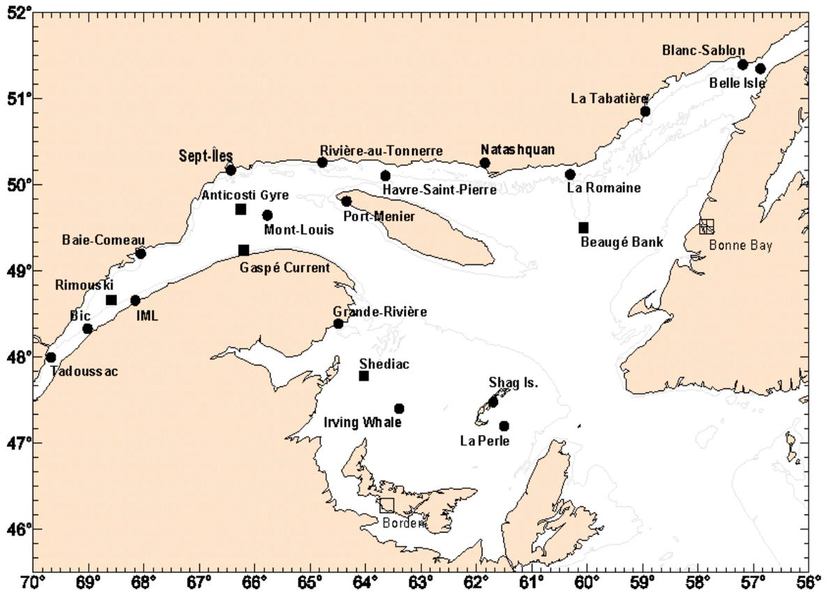
Figure 6. Locations of IML thermograph network stations in 2006, including regular stations where data are logged internally and recovered at the end of the season (circles) and oceanographic buoys that transmit data in real-time (solid squares). Locations for Borden and Bonne Bay are also shown (open squares) although they are no longer occupied.
