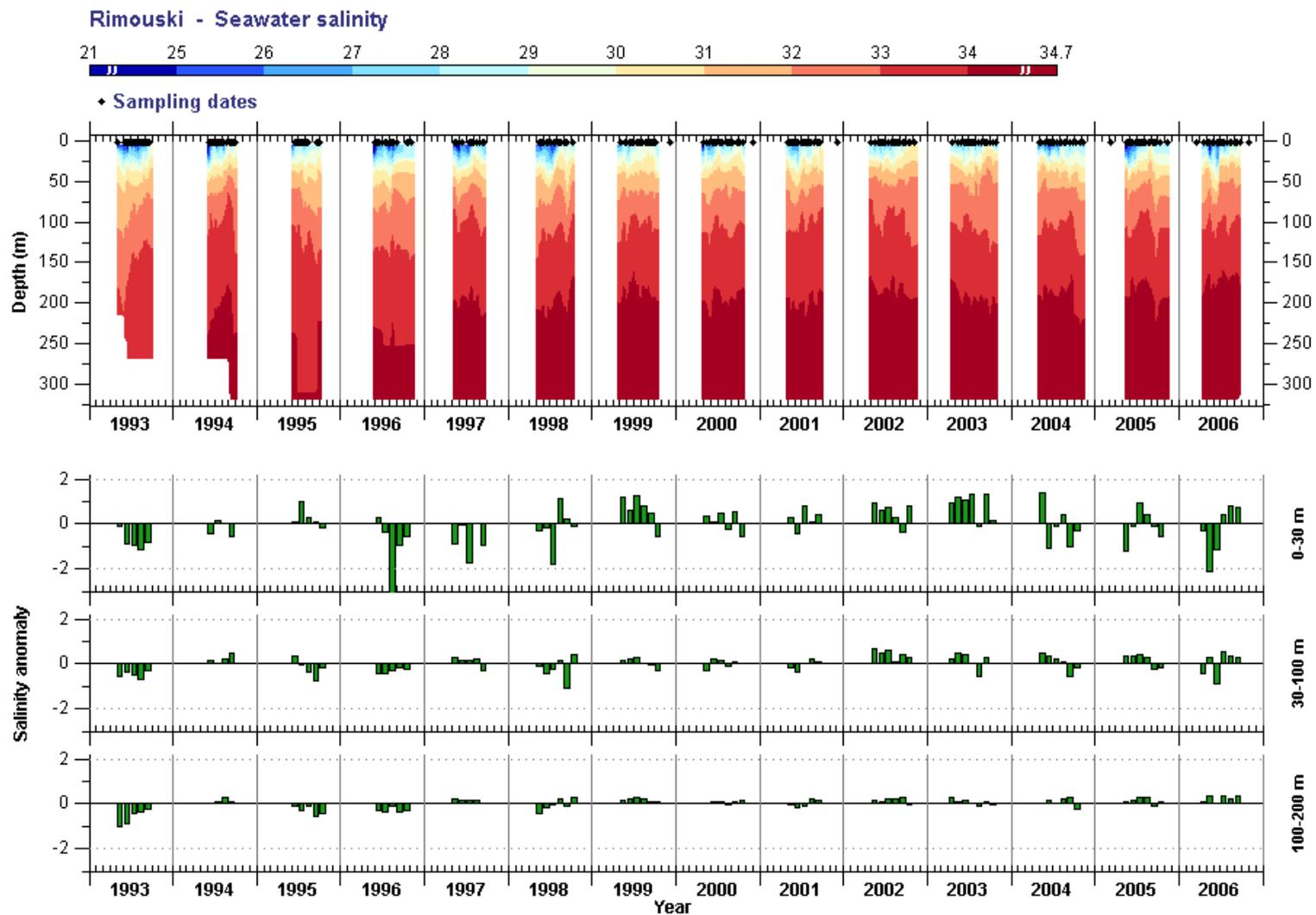
Figure 33. Isohaline time-series at the Rimouski station (top panel) and temperature anomaly by depth layers (lower panel).
