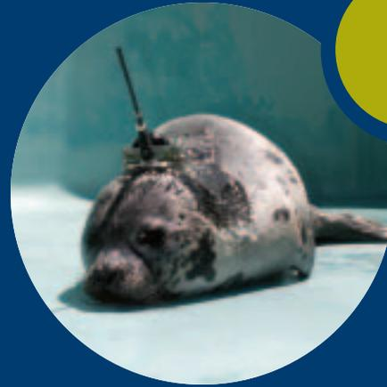
Harp seal with satellite tag on top of the head. The seal will shed the tag during its annual moult. This tag measures temperature and depth of water. This information and location is relayed via satellite. Photo Credit: DFO Newfoundland
