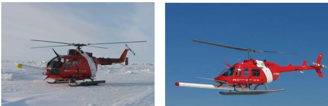
Figure 2: IcePic™ installed on MBB BO105 (left) and Bell 206L (right) helicopters
