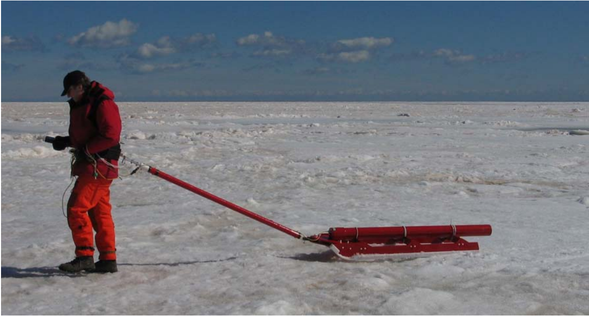
Figure A-1: Surface Ice Sensor™ system in operation on ice in the Northumberland Strait south of Prince Edward Island.
