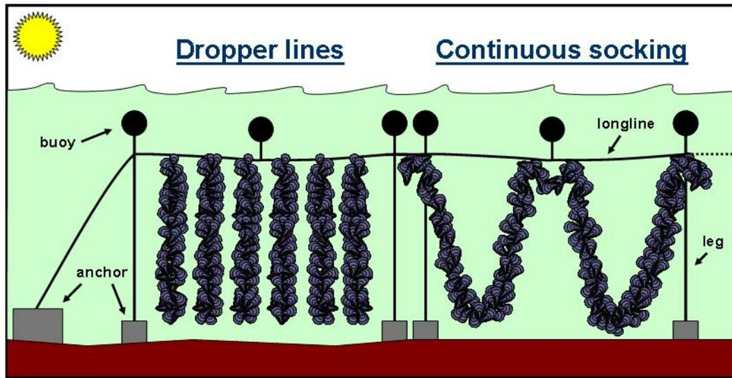
Figure 1. Schematic of a basic mussel longline system. The two most common systems used in Canada are shown. Longline systems may also be used for the culture of other species in nets, trays, etc.
