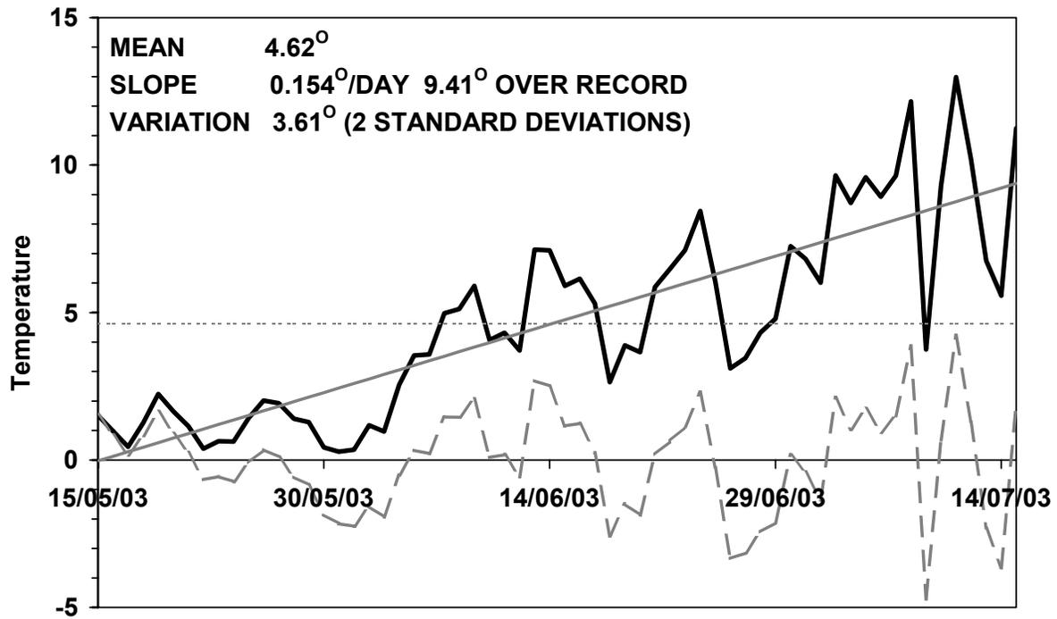
Figure 6. The temperature record from LFA27, 22.3 m in 2003 (solid black line), the mean (grey, dotted line), the linear trend (solid grey line) and residual (temperature with mean and trend removed; grey, long dashed line) over the record.
