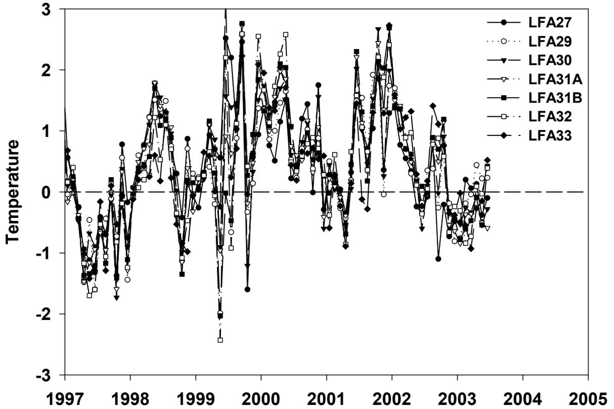
Figure 3. Time series of sea surface temperature anomalies 1997-2003 derived from satellite observations. The anomalies are obtained by subtracting the long-term mean (1985-2003) from the actual measurements.
