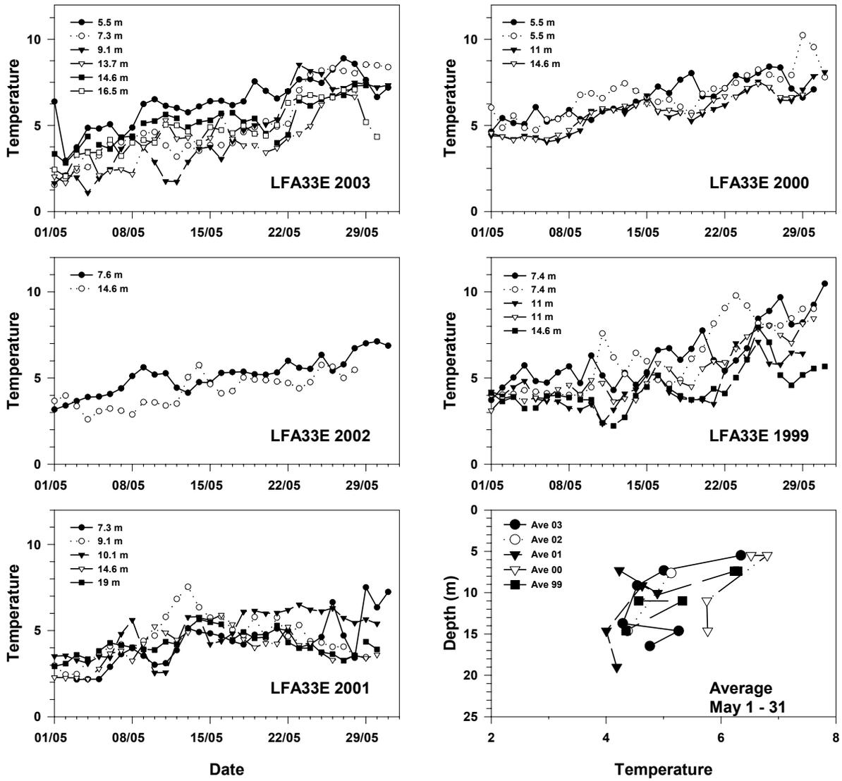
Figure 18. Time series of daily temperatures for LFA33E for 1999-2003 spring period at depths indicated in the legends. The depth profile of average temperatures is also shown.
