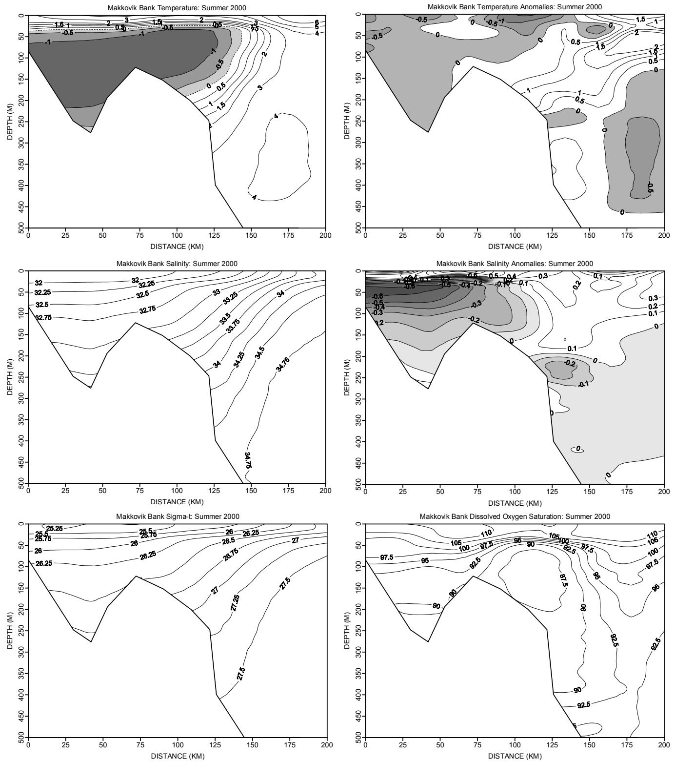
Fig. 23. Contours of temperature and salinity and their anomalies, sigma-t and dissolved oxygen saturation along the Makkovik Bank transect during the summer of 2000.
