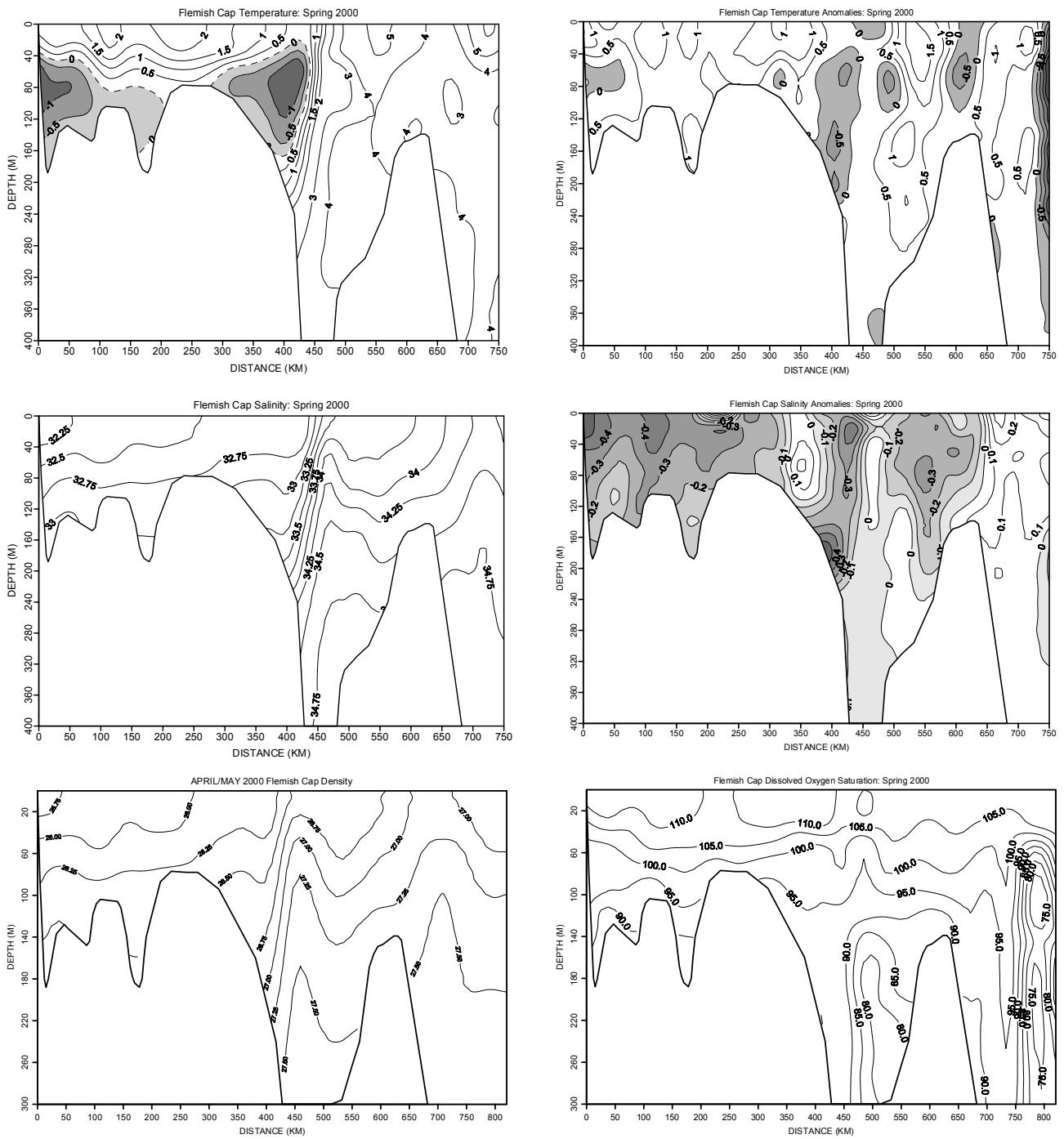
Fig. 15. Contours of temperature and salinity and their anomalies, sigma-t and dissolved oxygen saturation along the standard Flemish Cap transect during the spring of 2000.
