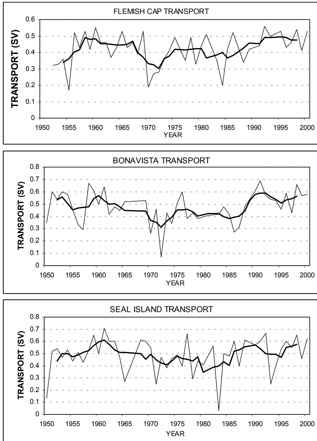
Fig. 29. Time series of geostrophic transport ( $10^6 \text{ m}^3/\text{s}$ ) relative to 130-m depth of the offshore branch of the Labrador Current through the Seal Island, Bonavista and Flemish Cap transects.
