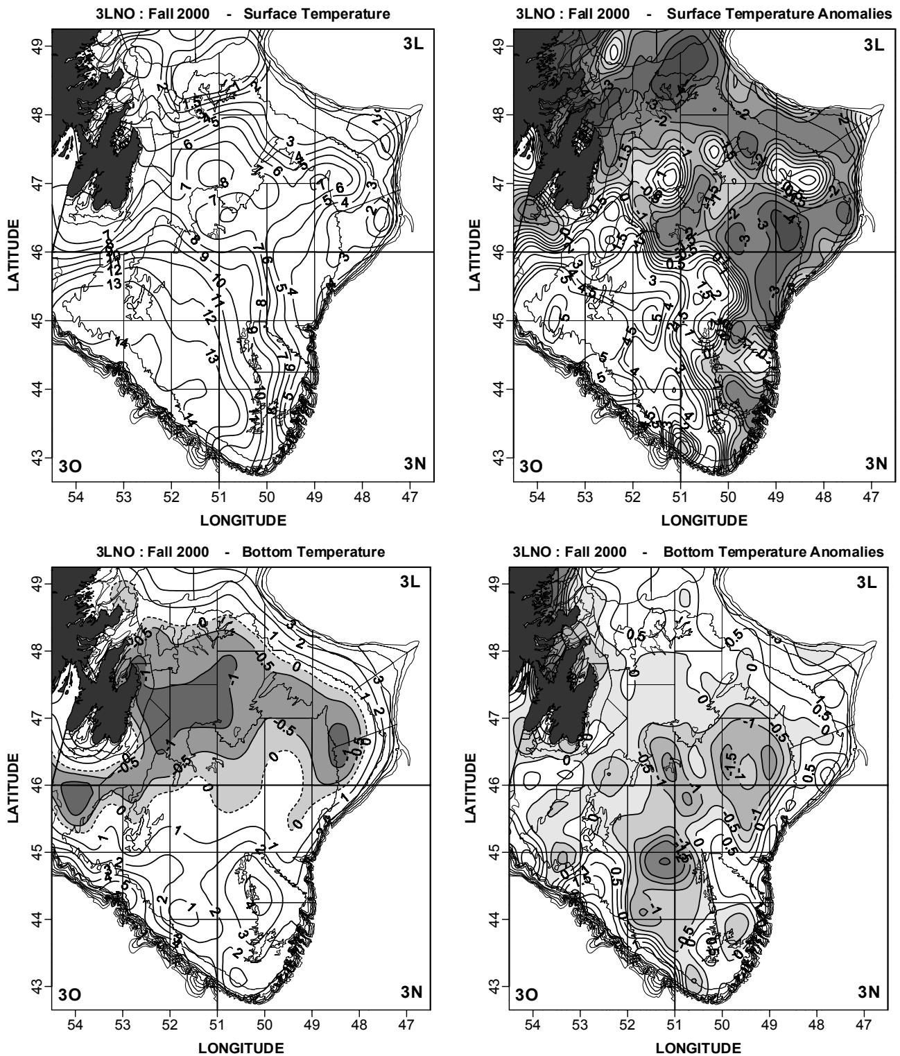
Fig. 32. Contours of surface and bottom temperature and their anomalies (in °C) for the fall of 2000 from the multi species survey of NAFO Divs. 3LNO.
