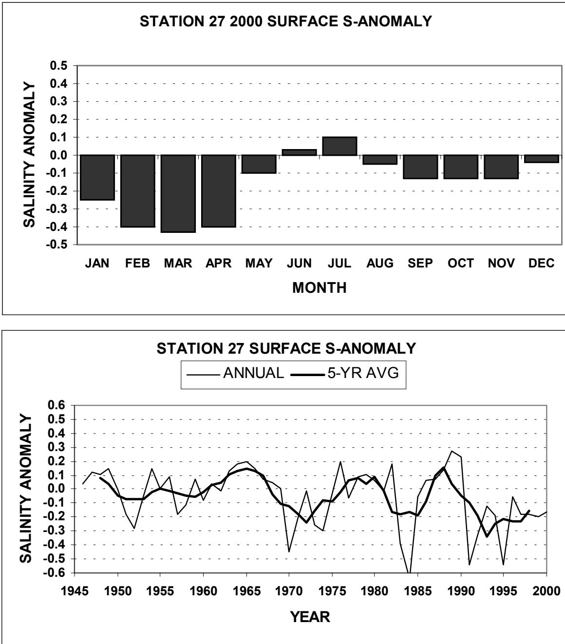
Fig. 5. Monthly surface salinity anomalies at Station 27 during 2000 (top) and the annual surface salinity anomalies and their 5-year running means (bottom).
