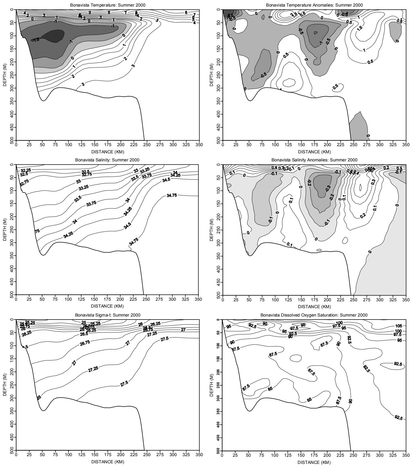
Fig. 19. Contours of temperature and salinity and their anomalies, sigma-t and dissolved oxygen saturation along the standard Bonavista transect during the summer of 2000.
