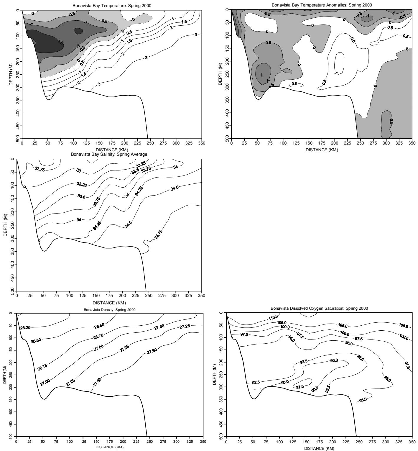
Fig. 18. Contours of temperature and temperature anomalies, salinity, sigma-t and dissolved oxygen saturation along the standard Bonavista transect during the spring of 2000. There were insufficient salinity data during this time period to produce a reliable average.
