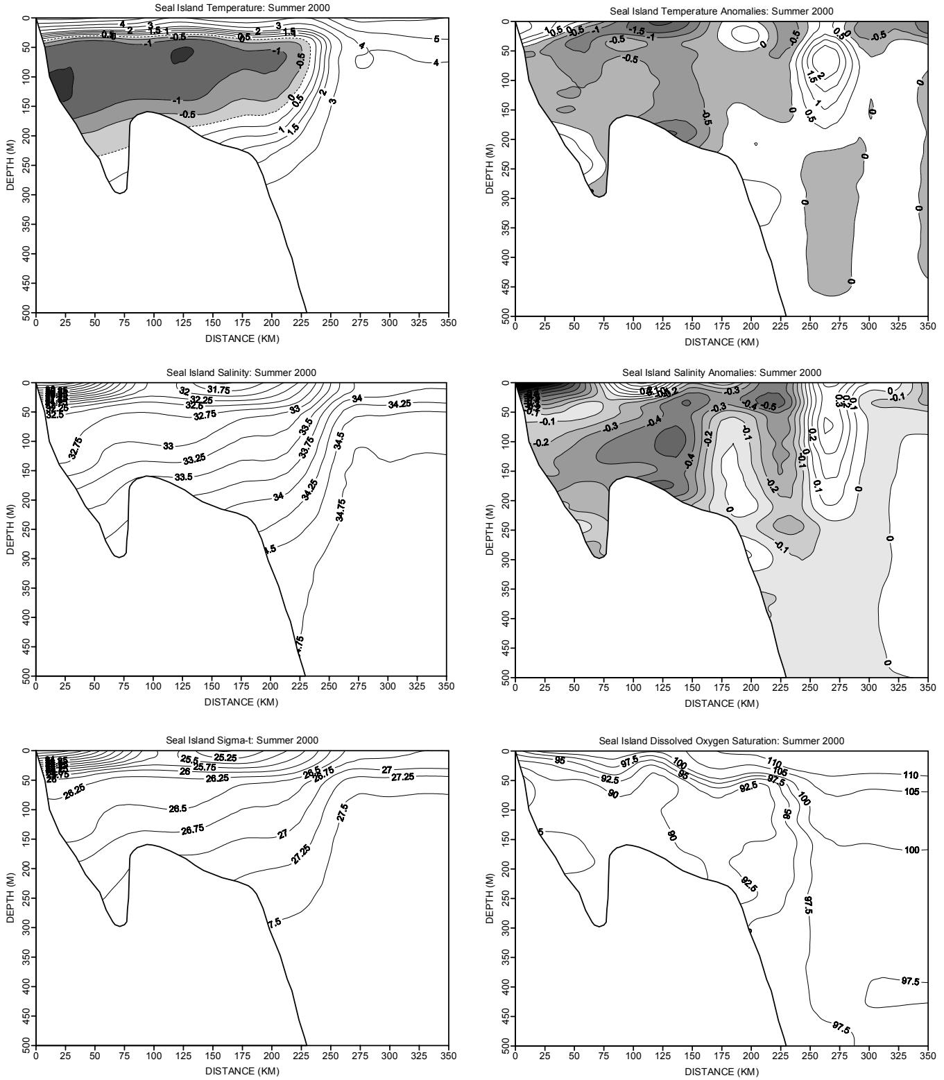
Fig. 22. Contours of temperature and salinity and their anomalies, sigma-t and dissolved oxygen saturation along the standard Seal Island transect during the summer of 2000.
