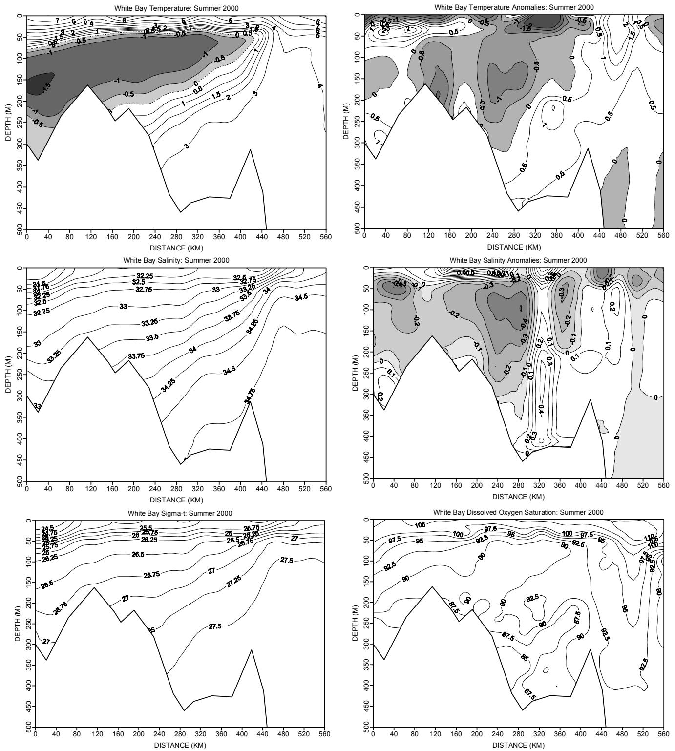
Fig. 21. Contours of temperature and salinity and their anomalies, sigma-t and dissolved oxygen saturation along the standard White Bay transect during the summer of 2000.
