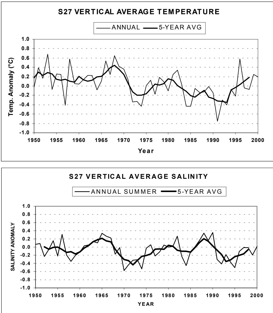
Fig. 7. The annual vertically averaged (0-176 m) Station 27 temperature anomalies and the vertically averaged (0-50 m) summer (July-Sept.) Station 27 salinity anomalies. The heavy lines are the 5-year running means.
