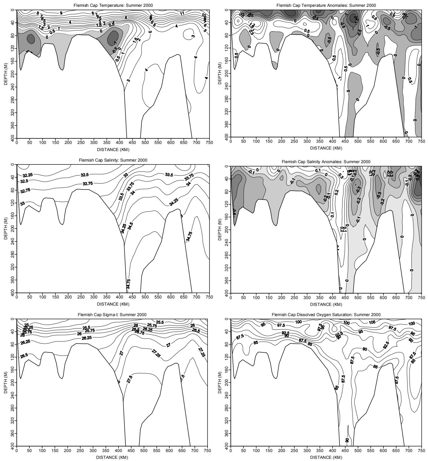
Fig. 16. Contours of temperature and salinity and their anomalies, sigma-t and dissolved oxygen saturation along the standard Flemish Cap transect during the summer of 2000.
