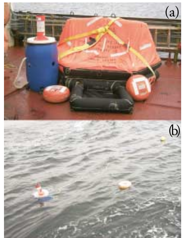
(a) Liferaft, Accurate Surface Tracker (AST) and two low-cost drifters (LCDs); (b) AST and LCD adrift at B1, trial #1.
