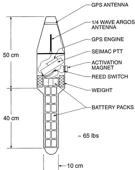
Fig. 2. Schematic of GPS-ARGOS beacon (redrawn from Seimac, 1995).
