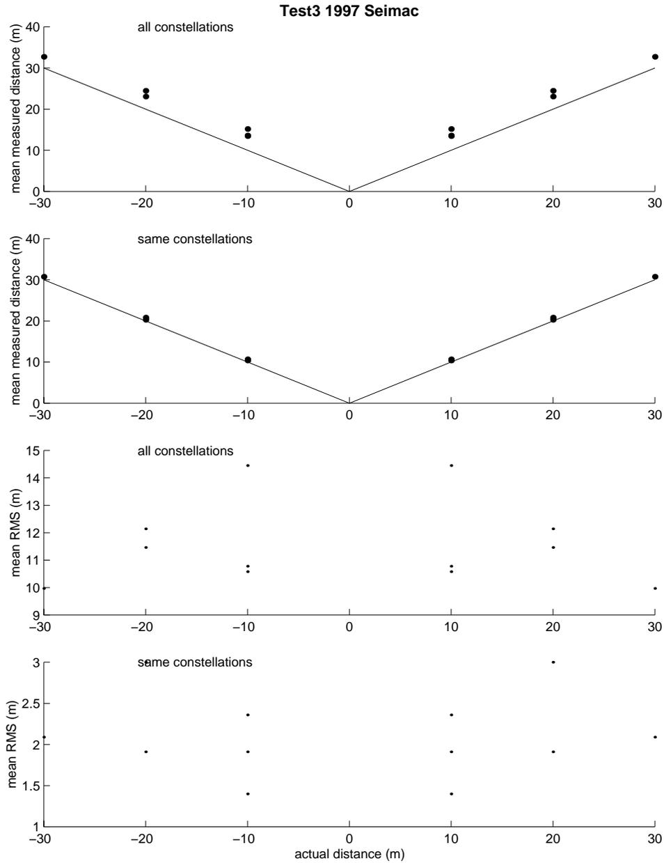
**Figure 12** Scatterplots of mean measured distance between beacons vs. actual distance between beacons and of mean RMS of measured distance between beacons vs. actual distance. Plots are shown for Test 3 in 1997 of type I Seimac beacons for when all observed satellites were used to obtain fixes and for when the two beacons observed the same satellite constellations.
