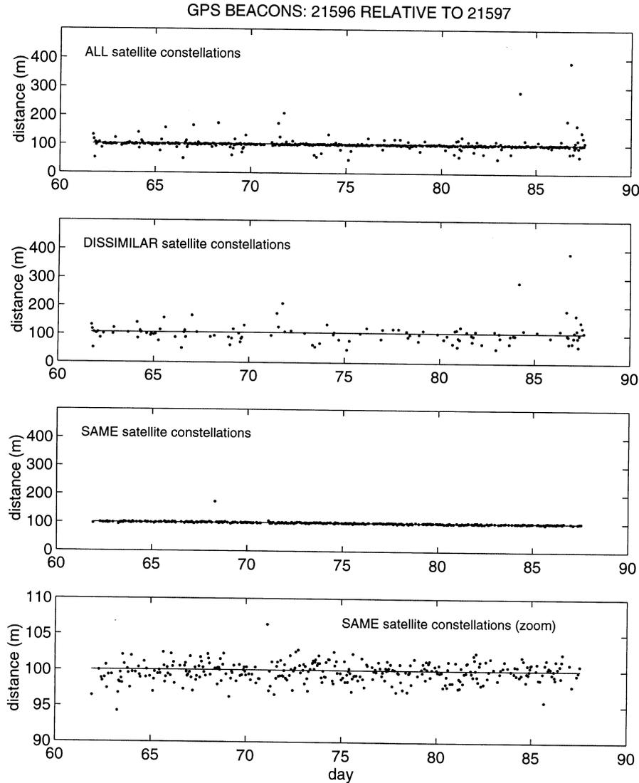
Fig. 4. Relative distance time series between beacons forming the southern corners of the 100 m  $\times$  100 m square.
