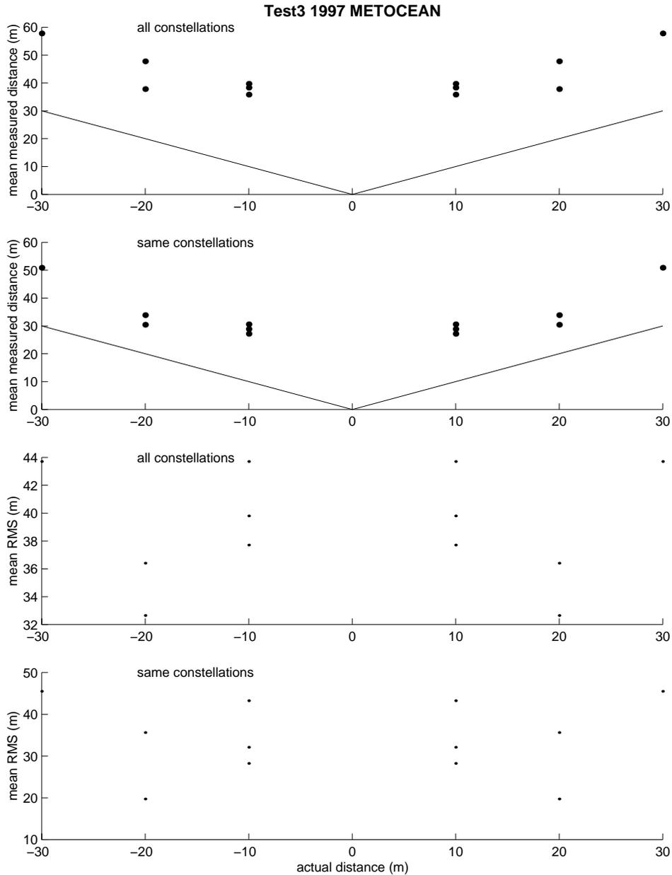
**Figure 13 Scatterplots of mean measured distance between beacons vs. actual distance between beacons and of mean RMS of measured distance between beacons vs. actual distance. Plots are shown for Test 3 in 1997 of type I METOCEAN beacons for when all observed satellites were used to obtain fixes and for when the two beacons observed the same satellite constellations.**
