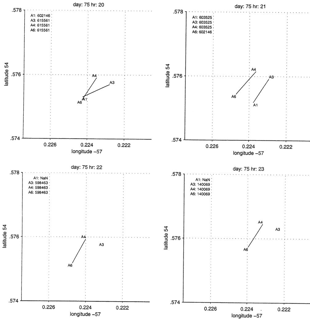
Fig. 6. Four consecutive snapshots of corners of the square when dissimilar satellite constellations are used for position fixes or when data is missing.
