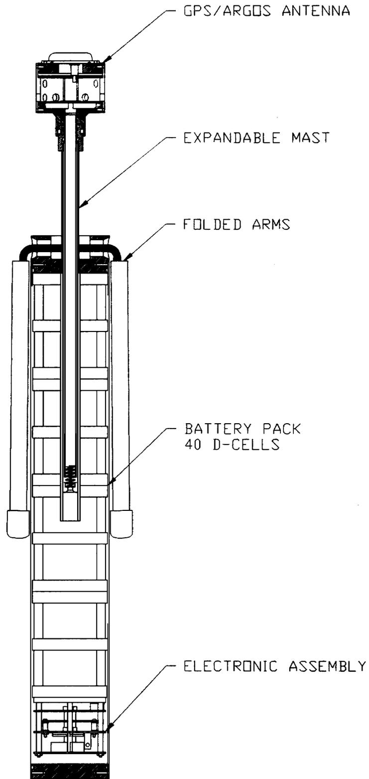
**Figure 4 Schematic diagram of 1997 METOCEAN, type I, location beacon (reproduced from METOCEAN, 1997).**
