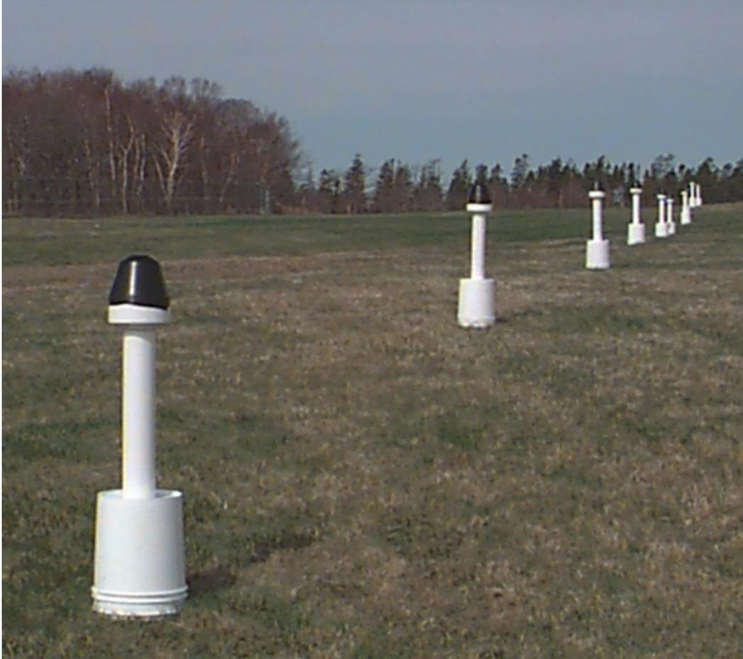
**Figure 7 1998 Seimac beacons (type II) are placed in line for stationary testing. The beacons were anchored in plastic buckets.**
