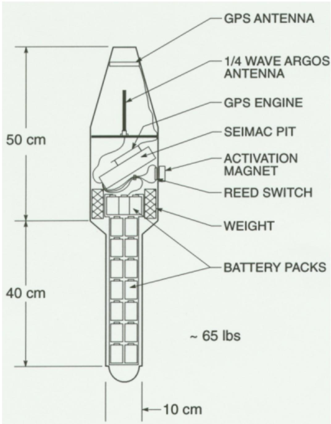
**Figure 2 Schematic diagram of 1997 Seimac (type I) GPS ice beacon (reproduced from Seimac, 1995).**
