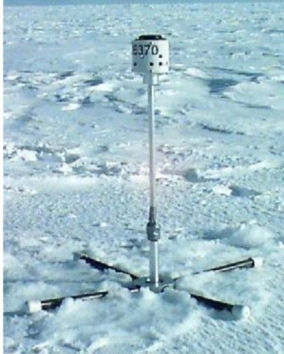
**Figure 3 Photo of 1997 METOCEAN GPS location beacon (type I).**
