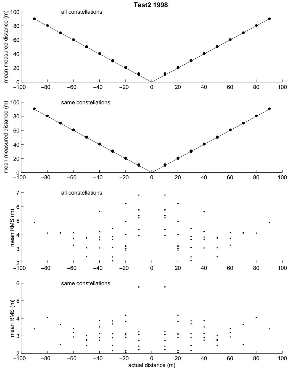
**Figure 16 Scatterplots of mean measured distance between beacons vs. actual distance between beacons and of mean RMS of measured distance between beacons vs. actual distance. Plots are shown for Test 2 in 1998 of type II METOCCEAN beacons for when one beacon was dropped from data analysis.**
