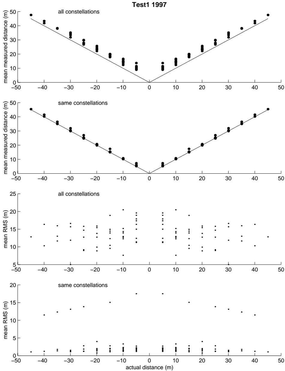
**Figure 9** Scatterplots of mean measured distance between beacons vs. actual distance between beacons and of mean RMS of measured distance between beacons vs. actual distance. Plots are shown for Test 1 in 1997 of type I Seimac beacons for when all observed satellites were used to obtain fixes and for when the two beacons observed the same satellite constellations.
