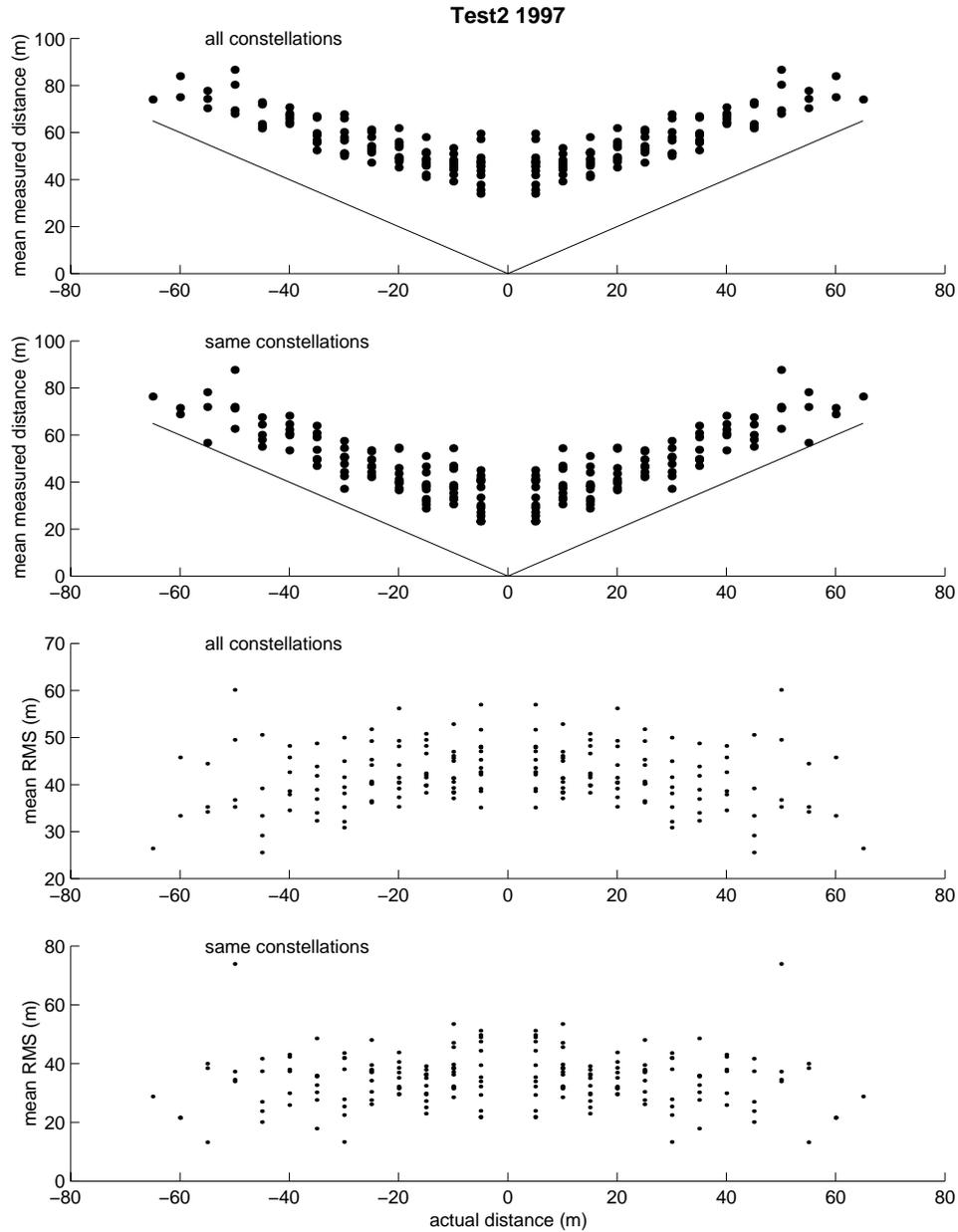
**Figure 11 Scatterplots of mean measured distance between beacons vs. actual distance between beacons and of mean RMS of measured distance between beacons vs. actual distance. Plots are shown for Test 2 in 1997 of type I METOCEAN beacons for when all observed satellites were used to obtain fixes and for when the two beacons observed the same satellite constellations.**
