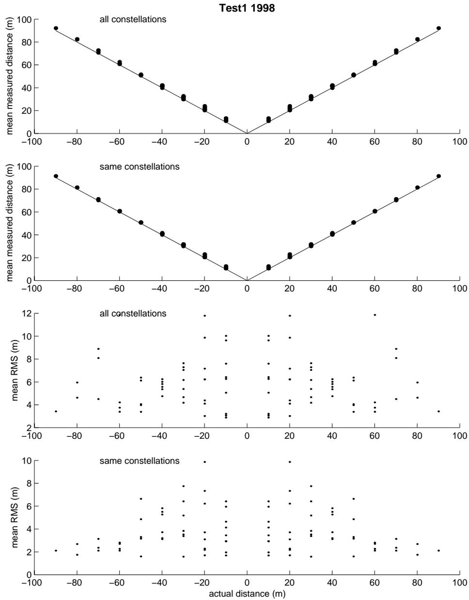
**Figure 14** Scatterplots of mean measured distance between beacons vs. actual distance between beacons and of mean RMS of measured distance between beacons vs. actual distance. Plots are shown for Test 1 in 1998 of type II METOCEAN beacons for when all observed satellites were used to obtain fixes and for when the two beacons observed the same satellite constellations.
