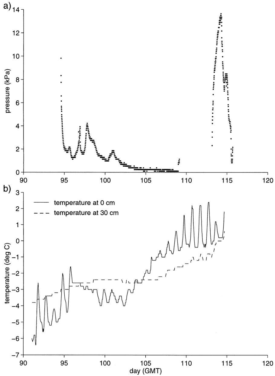
Fig. 7. Time series of ice pressure, ice temperature (30 cm) and ice/air interface temperature (0 cm) from the middle of a 250 m  $\times$  200 m ice floe, 60 cm thick.
