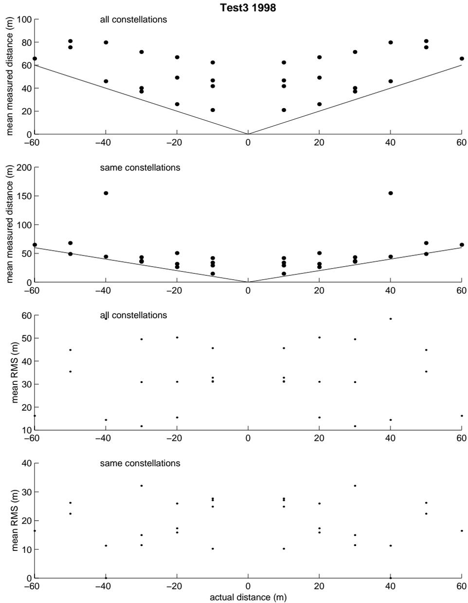
**Figure 17 Scatterplots of mean measured distance between beacons vs. actual distance between beacons and of mean RMS of measured distance between beacons vs. actual distance. Plots are shown for Test 3 in 1998 of type I METOCEAN beacons for when all observed satellites were used to obtain fixes and for when the two beacons observed the same satellite constellations.**
