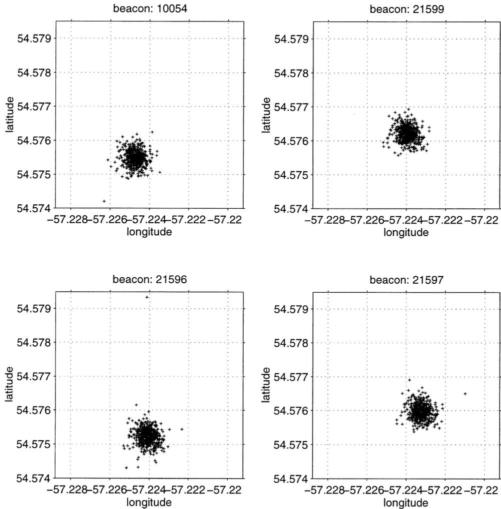
Fig. 3. Scatter plots of hourly position data from four GPS-ARGOS beacons forming a 100 m  $\times$  100 m square in the coastal land-fast ice rubble.
