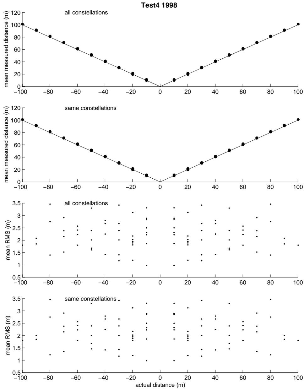
**Figure 19** Scatterplots of mean measured distance between beacons vs. actual distance between beacons and of mean RMS of measured distance between beacons vs. actual distance. Plots are shown for Test 2 in 1998 of type II beacons for when one beacon was dropped from data analysis.
