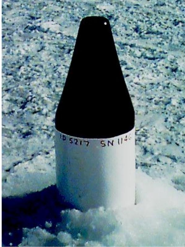
**Figure 1 Photo of 1997 Seimac GPS location beacon (type I).**
