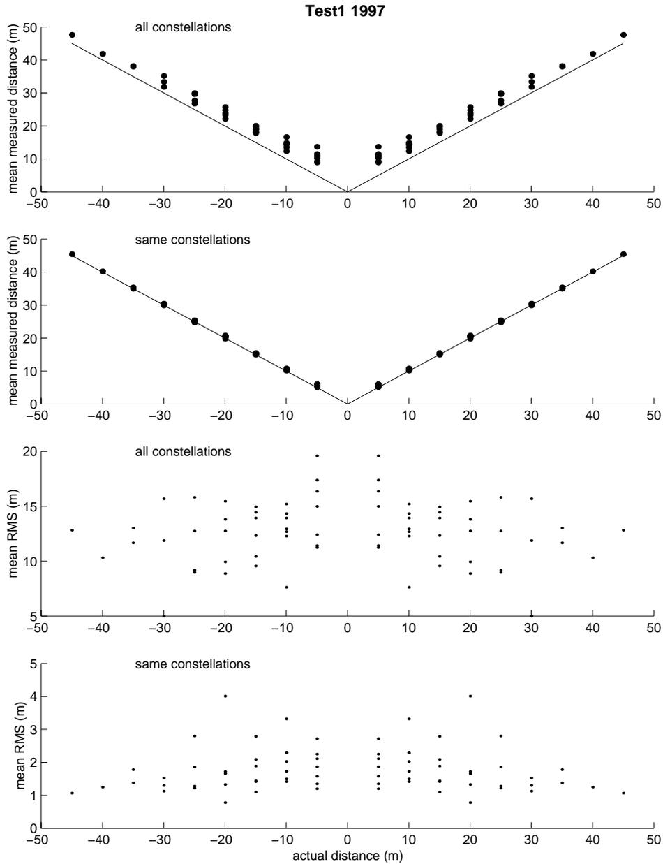
**Figure 10** Scatterplots of mean measured distance between beacons vs. actual distance between beacons and of mean RMS of measured distance between beacons vs. actual distance. Plots are shown for 9 type I Seimac beacons in Test 1 in 1997 for when all observed satellites were used to obtain fixes and for when the two beacons observed the same satellite constellations. The outliers evident in Figure 9 no longer exist.
