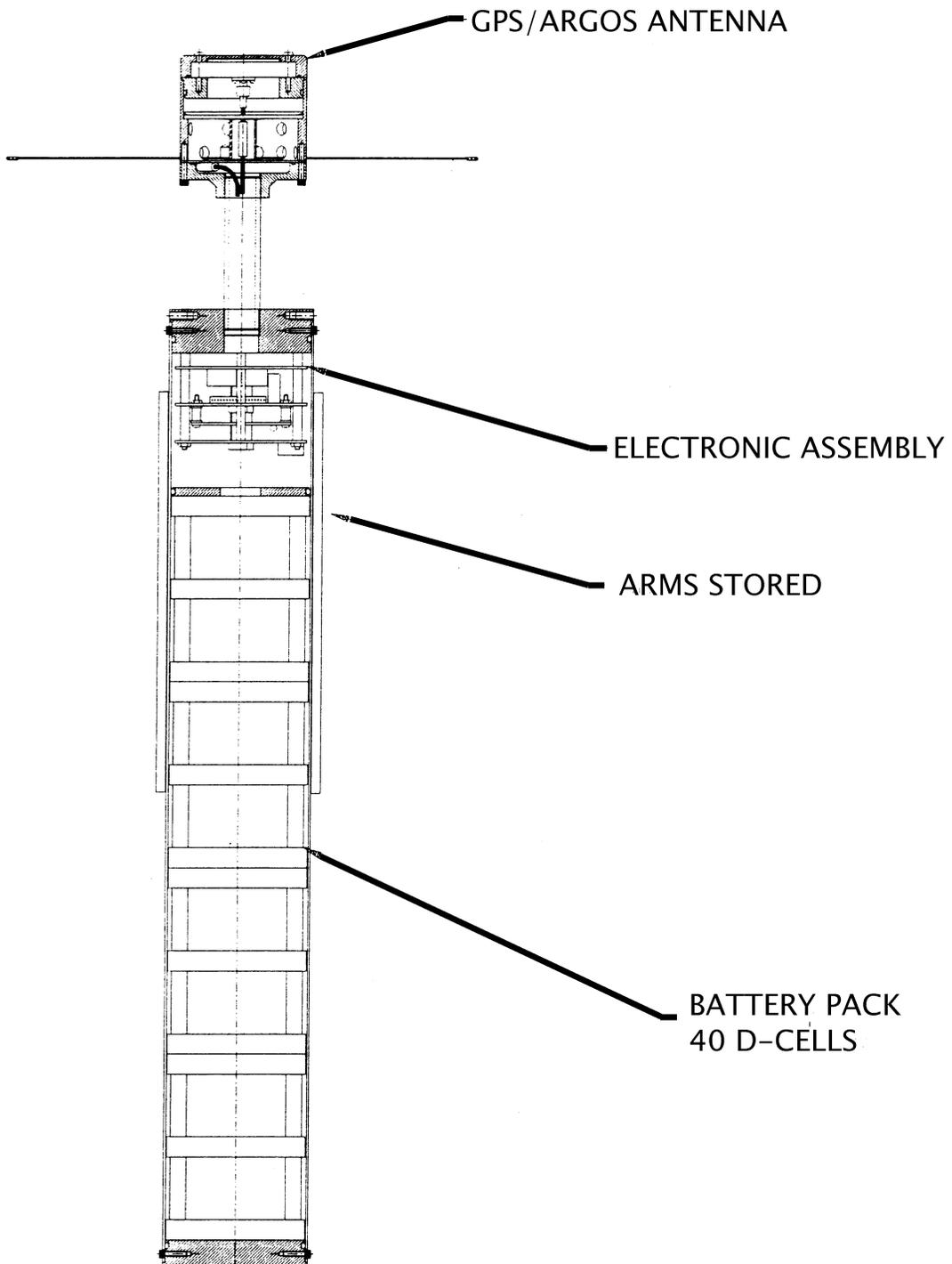
**Figure 6 Diagram of 1998 (type II) METOCEAN GPS location beacon with non-expandable mast.**
