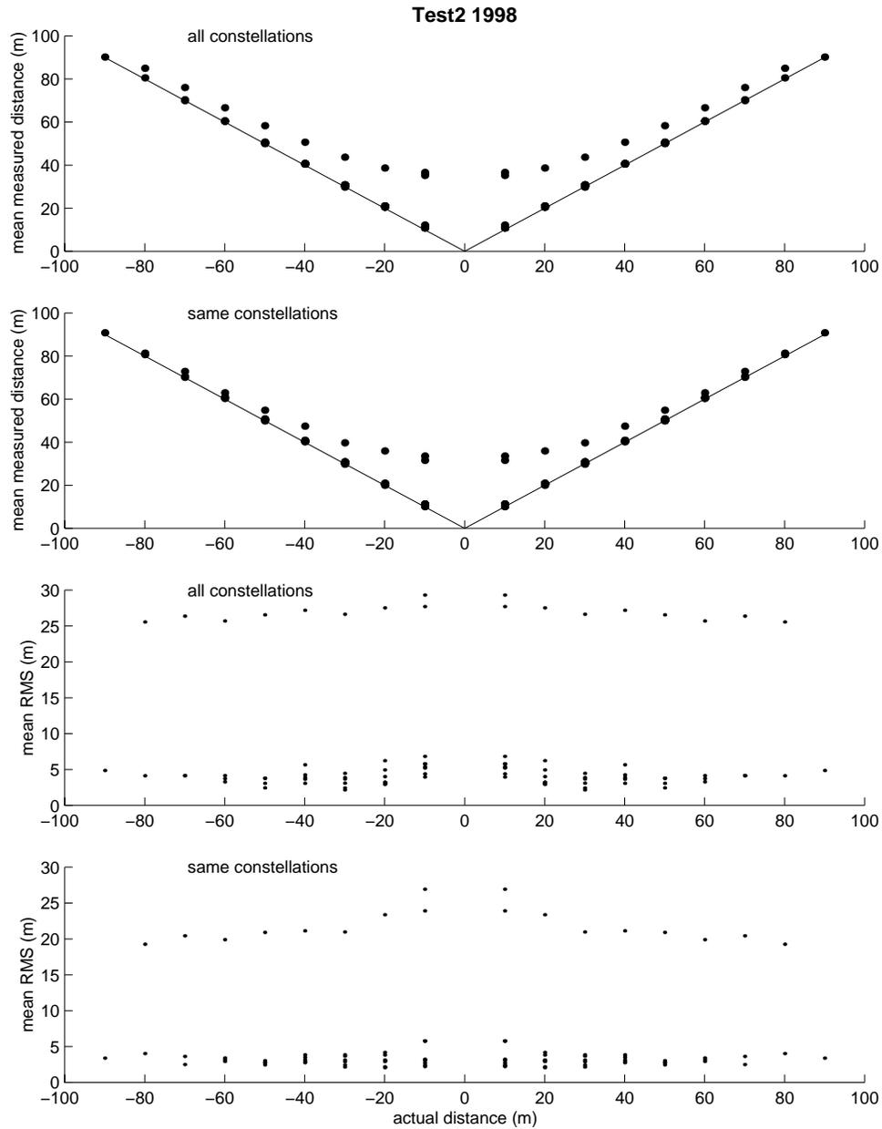
**Figure 15 Scatterplots of mean measured distance between beacons vs. actual distance between beacons and of mean RMS of measured distance between beacons vs. actual distance. Plots are shown for Test 2 in 1998 of type II METOCEAN beacons for when all observed satellites were used to obtain fixes and for when the two beacons observed the same satellite constellations.**
