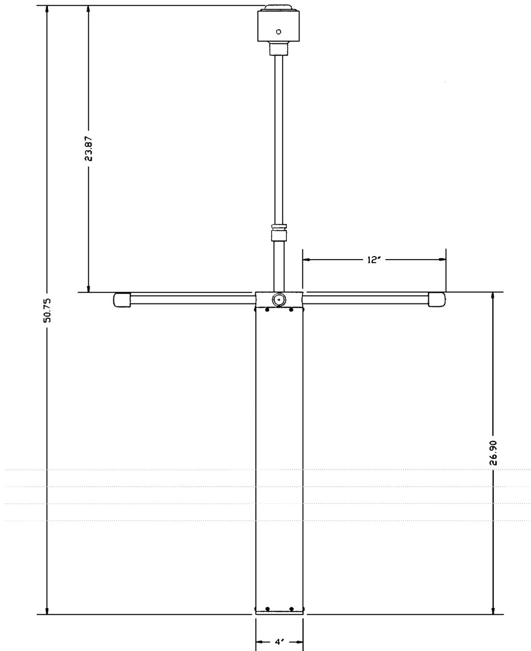
**Figure 5 Diagram of deployed 1997 METOCEAN, type I, GPS location beacon (reproduced from METOCEAN, 1997).**
