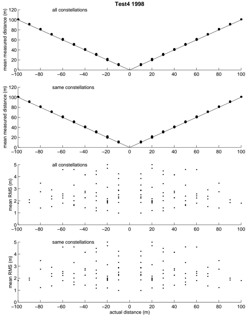
**Figure 18** Scatterplots of mean measured distance between beacons vs. actual distance between beacons and of mean RMS of measured distance between beacons vs. actual distance. Plots are shown for Test 4 in 1998 of type II beacons for when all observed satellites were used to obtain fixes and for when the two beacons observed the same satellite constellations.
