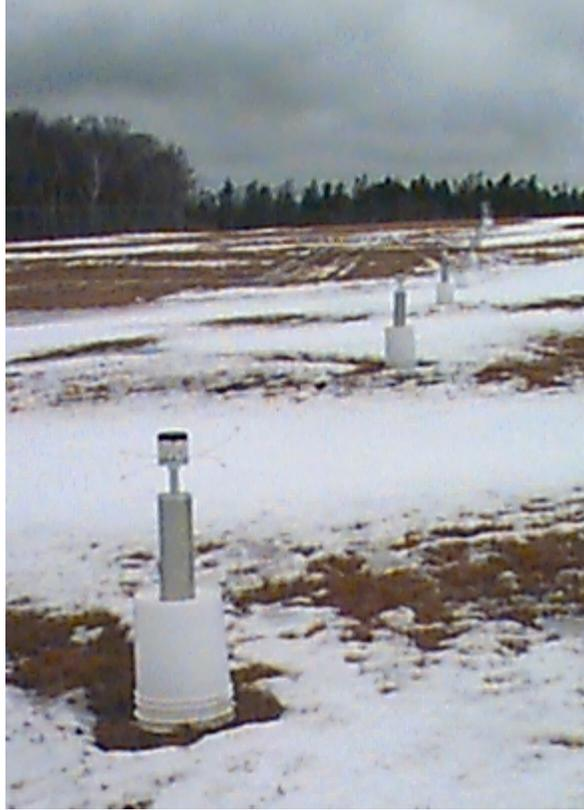
**Figure 8 1998 METOCEAN beacons (type II) in line for stationary tests. The beacons were anchored in plastic buckets.**
