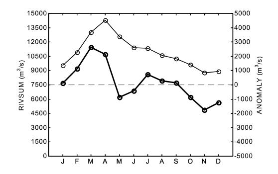
Fig. 10. Sum of the monthly averaged freshwater discharges of the St. Lawrence, Ottawa and Saguenay Rivers from January to December 1998 (RIVSUM index, thin line, left scale). The deviations with respect to the 1961-1990 mean (anomalies) are indicated by the thick line (right scale).
