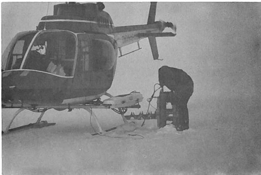
Figure A-4: Flushing of CTD Probe before profiling.
