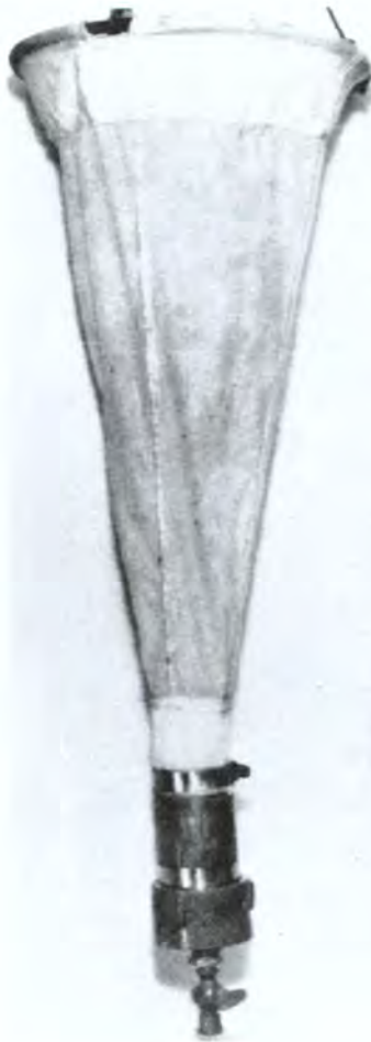
FIG. 41. Plankton net used in sampling oyster larvae. \times 0.2 .
