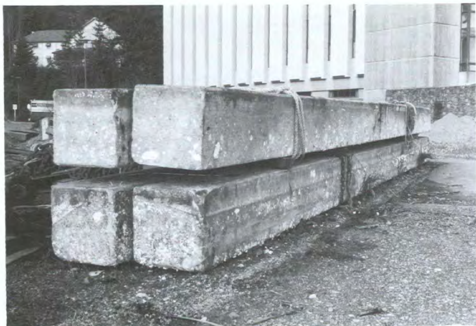
FIG. 119. Cement float logs.
